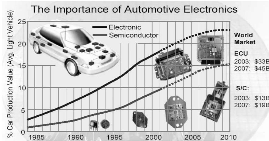
Figure 1.1: Percentage of the production value of an average light vehicle due to the semiconductors (lower curve) and due to the whole electronic systems (upper curve) vs. years (source: Bosch [1]).
