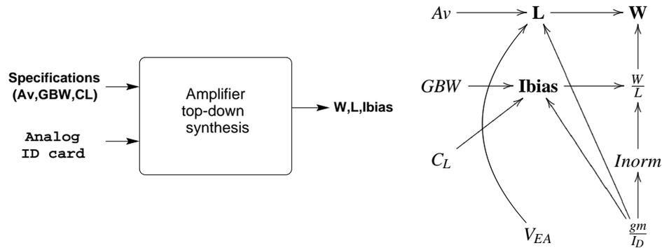
Figure 7.9: Top-down  $\frac{gm}{I_D}$  design methodology which takes the analog ID card as input and gives as result the transistor sizes ( $W, L$ ) and bias current ( $I_{bias}$ ).
