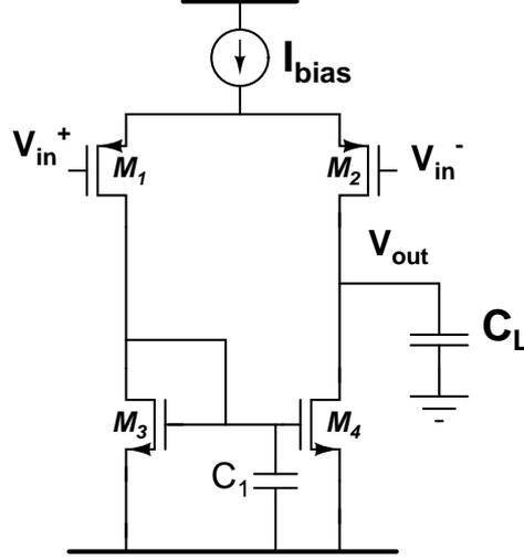
Figure 4.10: Current mirror included in an input stage of a two-stage amplifier biased by a DC current source ( $I_{bias}$ ) and loaded by a capacitance ( $C_L$ ).  $C_1$  is the parasitic capacitance associated to the mirror.
