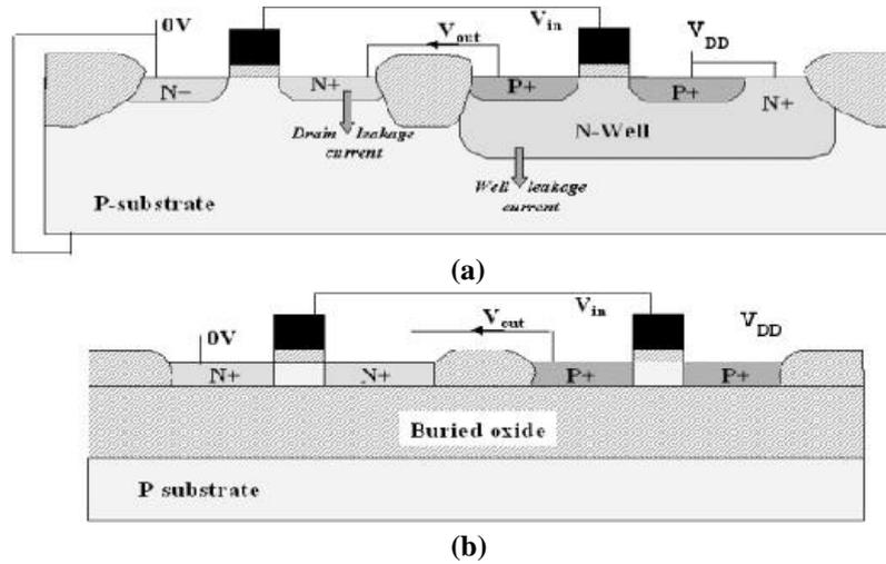
Figure 1.2: Cross-section of a CMOS inverter in a bulk (a) and in a silicon-on-insulator (b) technology [9].
