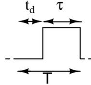
Figure 6.11: Generic feedback DAC return-to-zero pulse (RTZ).  $T$  is the sampling period,  $t_d$  is the pulse delay and  $\tau$  is the pulse width or duty cycle.
