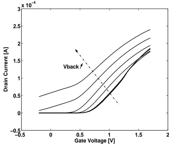
Figure A.1: Measured  $I_D$  vs.  $V_G$  corresponding to a back gate voltage ( $V_{back}$ ) varying from  $-40\text{ V}$  to  $40\text{ V}$  in  $10\text{ V}$  steps. nMOSFET low leakage with  $L = 0.5\ \mu\text{m}$  and  $W = 10\ \mu\text{m}$ ,  $V_D = 50\text{ mV}$  and  $V_S = 0\text{ V}$ .
