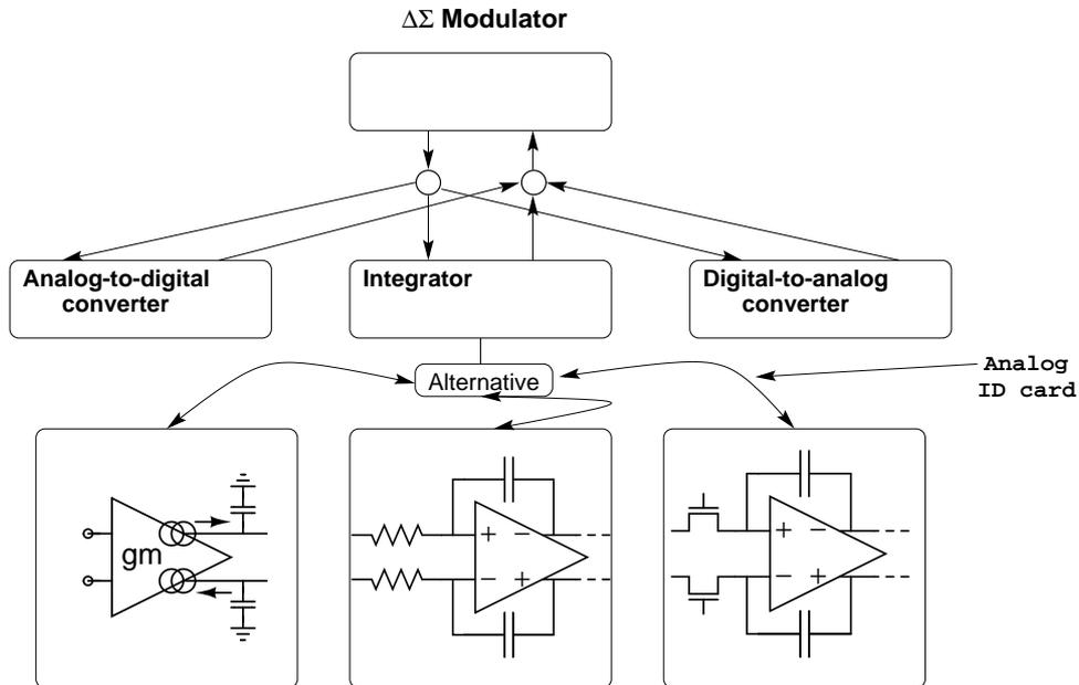
Figure 7.6: Top-down structural division of a  $\Delta\Sigma$  modulator with continuous-time integrators. Three subsystems are identified: integrator, analog-to-digital converter and digital-to-analog converter. We focus on the three different topologies for the integrators.
