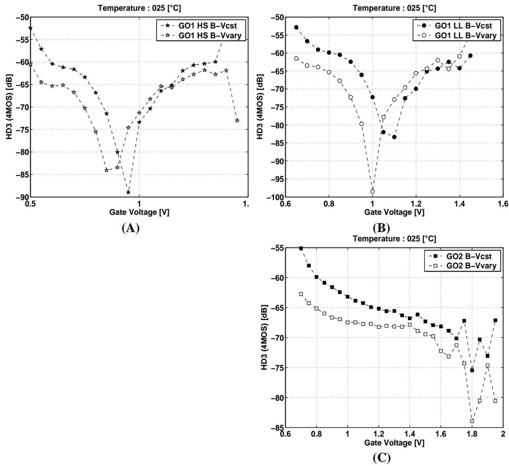
Figure B.3: HD3[dB] vs.  $V_G$  for 4-MOS structures composed of devices GO1 HS (thin-gate oxide, low  $V_{th}$ )(A), GO1 LL (thin-gate oxide, high  $V_{th}$ )(B) and GO2 (thick-gate oxide) (C) with body connected to the fixed potential terminal (full symbols) and with body connected to the varying signal source (void symbols). All devices are  $10\ \mu\text{m}$  long and  $10\ \mu\text{m}$  large.  $V_a = 200\ \text{mV}$  around  $V_o = 0\ \text{V}$ , at room temperature.
