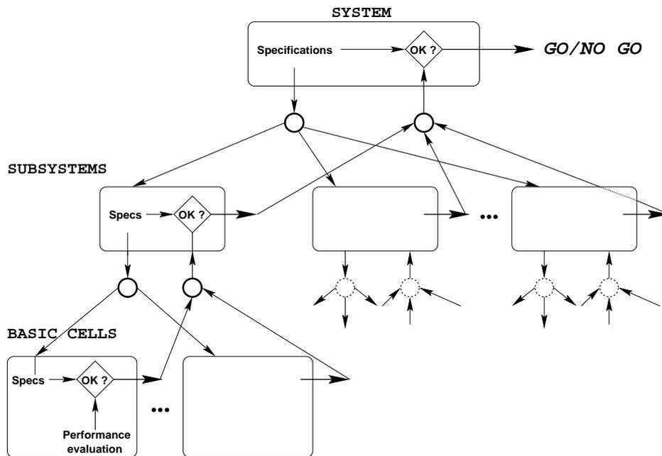
Figure 7.4: Guided top-down design and bottom-up validation flows of analog circuits using HDL-AMS. The specifications are downwards propagated to the different subsystems while the performance of these subsystems are aggregated to verify locally if the performance and specifications are adequate [9].
