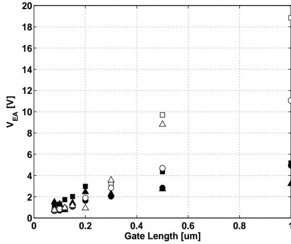
Figure 2.8: Measured  $V_{EA}$  at  $I_{norm} = 4 \mu A$  vs. gate length for n-type MOSFETs of Bulk ( $\square$ ), FD SOI ( $\circ$ ) and PD SOI ( $\triangle$ ) transistors. Each device type with (full symbols) and without HALO implantation (void symbols).  $W = 10 \mu m$  for all devices,  $L_{nom} = 0.12 \mu m$ ,  $V_D = 0.50 V$  and  $V_S = 0 V$ .
