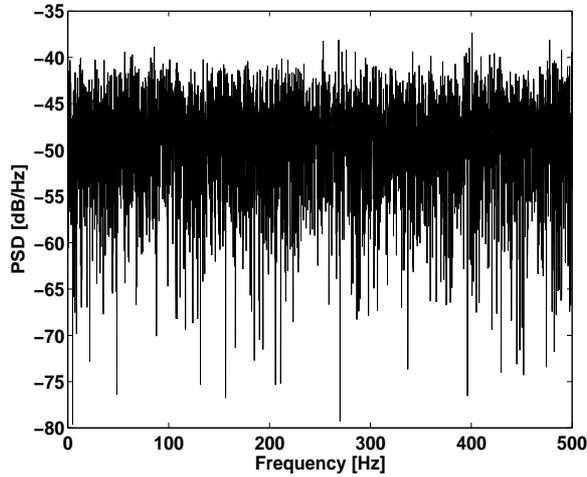
Figure 5.17: Power spectral density [dB/Hz] vs. frequency [Hz] of the noise samples generated using VHDL-AMS entity *wn\_source* with  $F_{smp} = 1$  kHz and  $PSD_{dB/Hz} = -50.0$  dB/Hz.
