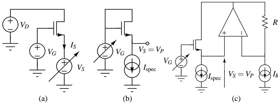
**Figure D.2:** Configuration for the measurement of (a)  $I_S$  vs.  $V_S$  and extraction of  $I_{\text{spec}}$ ; (b)  $V_P$  vs.  $V_G$ ; and (c)  $V_P$  vs.  $V_G$  for short-channel transistors.
