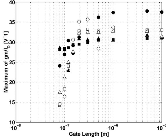
Figure 2.7: Maximum of measured  $\frac{gm}{I_D}$  ratio vs. gate length for n-type MOSFETs of Bulk ( $\square$ ), FD SOI ( $\circ$ ) and PD SOI ( $\Delta$ ) transistors. Each device type with (full symbols) and without HALO implantation (void symbols).  $W = 10 \mu m$  for all devices,  $L_{nom} = 0.12 \mu m$ ,  $V_D = 0.75 V$  and  $V_S = 0 V$ .
