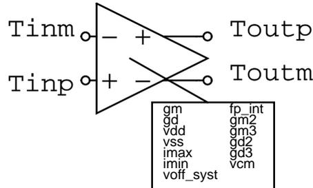
Figure 5.5: Schematic description of the entity corresponding to the fully-differential OTA. The ports are four terminals of electrical nature and the generics are of type real.
