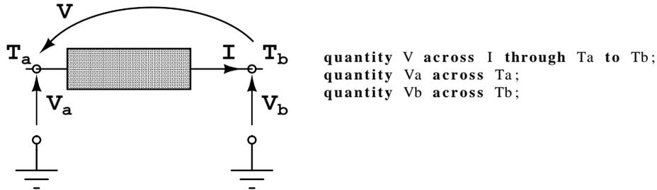
**Figure 5.4:** Branch across ( $V_a$ ,  $V_b$ ,  $V$ ) and through ( $I$ ) quantities associated to the terminals  $T_a$  and  $T_b$ . If the nature of the terminals are defined as electrical, then the across quantities are voltages and through quantities are currents. The reference (electrical ground) is intrinsically defined (see  $V_a$  and  $V_b$  declarations.)
