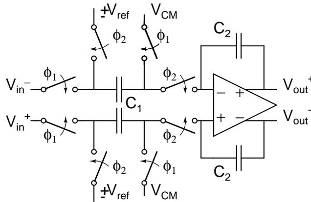
**Figure 6.7: Fully-differential switched-capacitor integrator.**  $\phi_1$  and  $\phi_2$  are non-overlapping clocks.  $V_{in}^+$  and  $V_{in}^-$  ( $V_{out}^+$  and  $V_{out}^-$ ) are the fully-differential inputs (outputs).  $V_{ref}$  is the feedback DAC output voltage and  $V_{CM}$  is the common-mode voltage.
