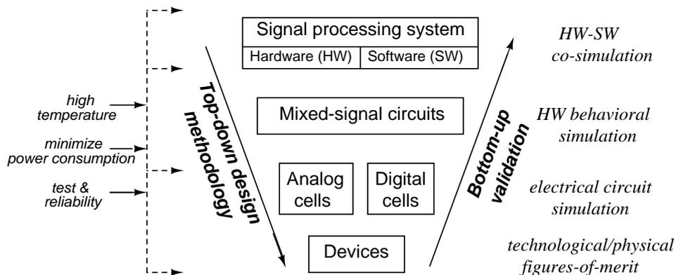
Figure 1.3: A signal processing system is divided into its subsystems: mixed-signal circuits, which are further divided into digital and analog circuits, both relying on devices. The different subsystems use different types of description and simulation protocols which must be linked in a hierarchical structure supporting top-down design and bottom-up validation.
