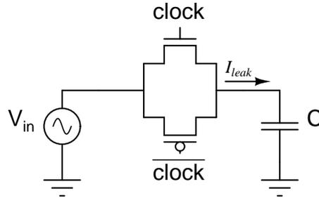
**Figure 6.8:** Transmission gate composed of a n-type and a p-type MOSFET's. n-type is driven by the clock signal (clock) and the p-type by its logic complement ( $\overline{\text{clock}}$ ).  $I_{leak}$  is the total leakage currents originating from the n and p-type MOSFETs.
