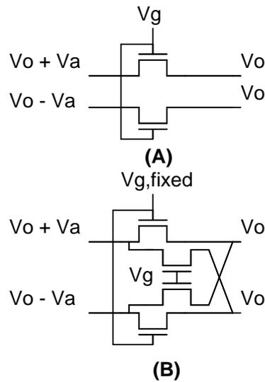
Figure 3.1: Resistive structures used in MOSFET-C filters to emulate tunable resistances: 2-MOS structure (A) [5] and 4-MOS Czarnul-Song structure (B) [7][8]
