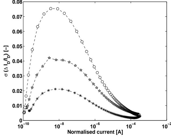
**Figure 4.2:** Measured  $\sigma_{(\Delta I_D/I_D)}$  [-] vs.  $I_{norm}$  [A] for n-type MOSFETs of a  $0.35 \mu\text{m}$  bulk CMOS technology for different device sizes:  $W = 40 \mu\text{m}$  and  $L = 10 \mu\text{m}$  (\*);  $W = 10 \mu\text{m}$  and  $L = 2 \mu\text{m}$  (★);  $W = 5 \mu\text{m}$  and  $L = 0.8 \mu\text{m}$  (○).  $V_D = 1.3 \text{ V}$ ,  $V_S = 0 \text{ V}$ .
