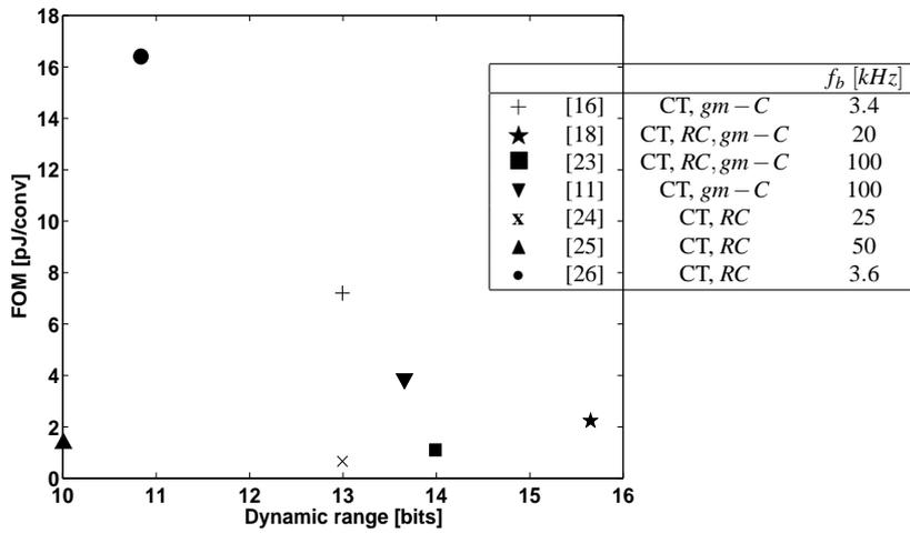
Figure 6.16: FOM [pJ/conv] vs. dynamic range [bits] of the published continuous-time (CT)  $\Delta\Sigma$  modulators targeting low to medium signal bandwidth ( $< 100\text{ kHz}$ ). [30] is not present to improve graph readability ( $FOM = 102.93$  [pJ/conv] for  $f_b = 72\text{ kHz}$  and  $DR = 8.66$  [bits]).
