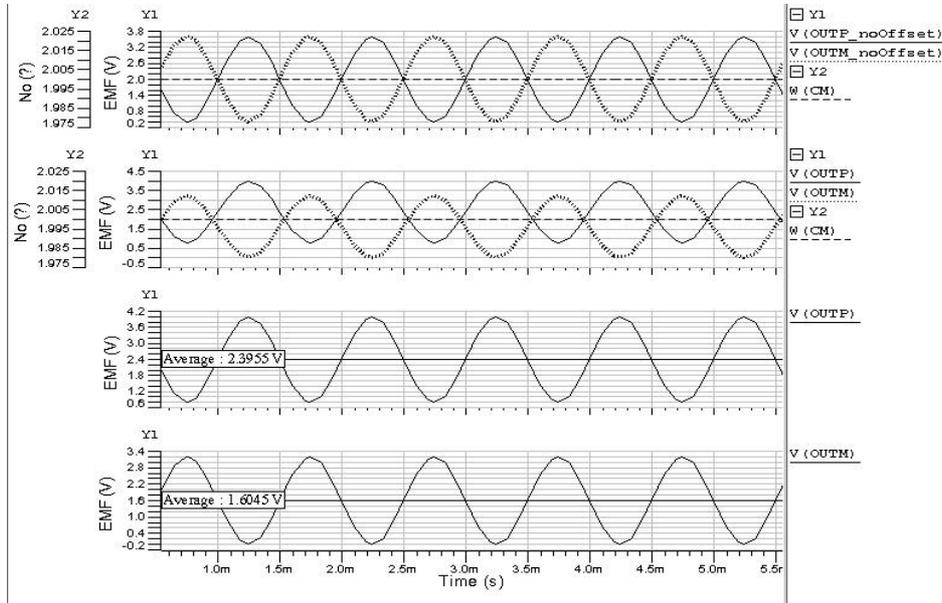
**Figure 5.12:** Output voltages [V] vs. time [s] of an OTA with a  $10mV$   $voff\_syst$  ( $Voutp$  and  $Voutm$ ) and with  $voff\_syst = 0$  V ( $VoutpnOffset$  and  $VoutmnOffset$ ).  $w(cm)$  is the common-mode output voltage [V].  $vcm = 2$  V,  $gm = 800 \mu S$  and  $gd = 10 \mu S$ , the OTA is loaded by a  $10$  pF capacitor.
