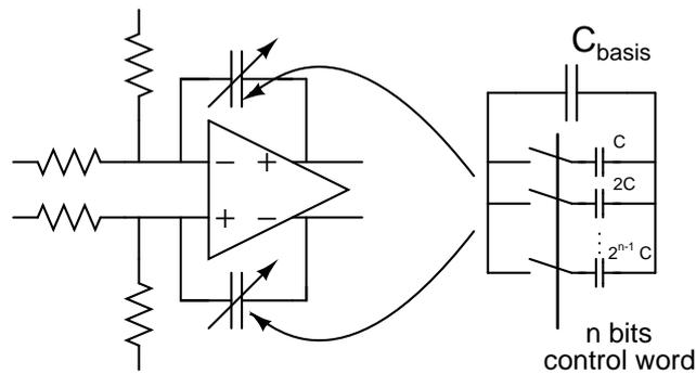
Figure 6.21: Discrete tuning of the capacitance for an active RC integrator. Algorithms to set up the  $n$ -bits control word can be found in [51][52][53]
