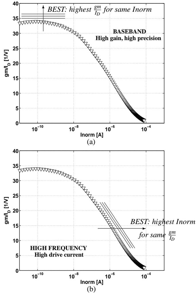
Figure 2.5: Measured  $\frac{g_m}{I_D}$  ratio vs.  $I_{norm}$  showing the different region of inversion corresponding to different types of application
