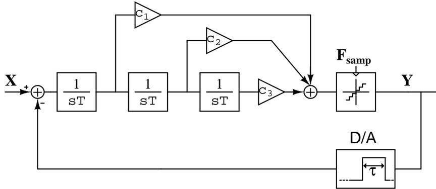
Figure 6.10: 3rd order CT  $\Delta\Sigma$  modulator stabilized by feedforward compensation.  $c_1$ ,  $c_2$  and  $c_3$  are the loop filter coefficients
