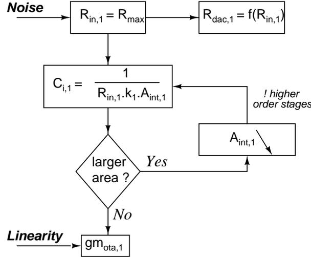
Figure 6.26: Design optimization methodology of the active RC integrators of a CT modulator supported by our VHDL-AMS models.
