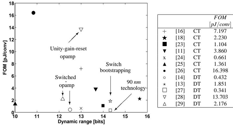
Figure 6.5: FOM [pJ/conv] vs. dynamic range [bits] of the published continuous-time (CT) and discrete-time (DT)  $\Delta\Sigma$  modulators targeting low to medium signal bandwidth ( $< 100\text{kHz}$ ). [30] (CT) is not present to improve graph readability ( $FOM = 102.93\text{ [pJ/conv]}$  for  $f_b = 72\text{ kHz}$  and  $DR = 8.66\text{ [bits]}$ ).
