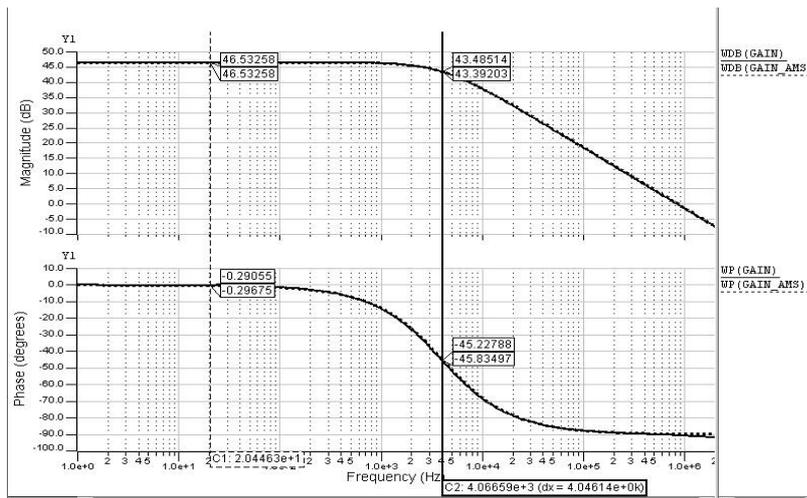
**Figure 5.13:** AC frequency responses in magnitude [dB] (up) and phase [°] (down) vs. frequency [Hz] for an OTA emulated by our model (dotted lines) and by a SPICE-like netlist (solid lines). The extracted OTA parameters are  $gm = 53.865 \mu S$ ,  $gd = 253.523$  nS and the OTA is loaded by a  $10$  pF capacitive load for both descriptions.
