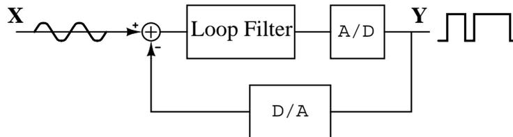
Figure 1.5: A modulator of a  $\Delta\Sigma$  analog-to-digital converter is composed of an analog loop filter, an internal analog-to-digital converter and a feedback digital-to-analog converter.
