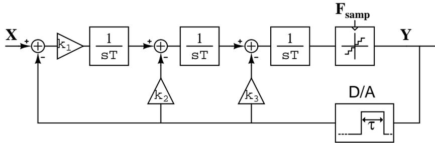
Figure 7.5: 3rd order  $\Delta\Sigma$  modulator with continuous-time integrators stabilized by feedback.  $k_1$ ,  $k_2$  and  $k_3$  are the loop filter coefficients
