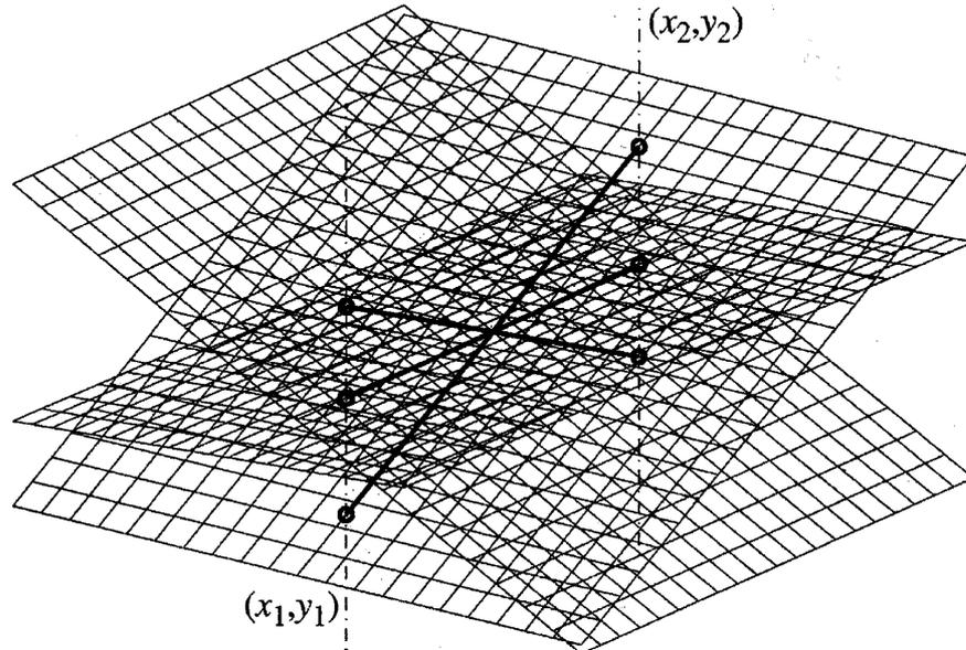
Figure C.1: The deterministic trend in the parameters value can be approximated by planes for small and medium sized dies [3]
