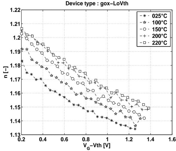
Figure 3.3: Linearized body effect factor ( $n$ ) in strong inversion [-] vs.  $V_G - V_{th}$  for gox-LoVth device at different temperatures.  $W = 10 \mu\text{m}$  and  $L = 10 \mu\text{m}$ .
