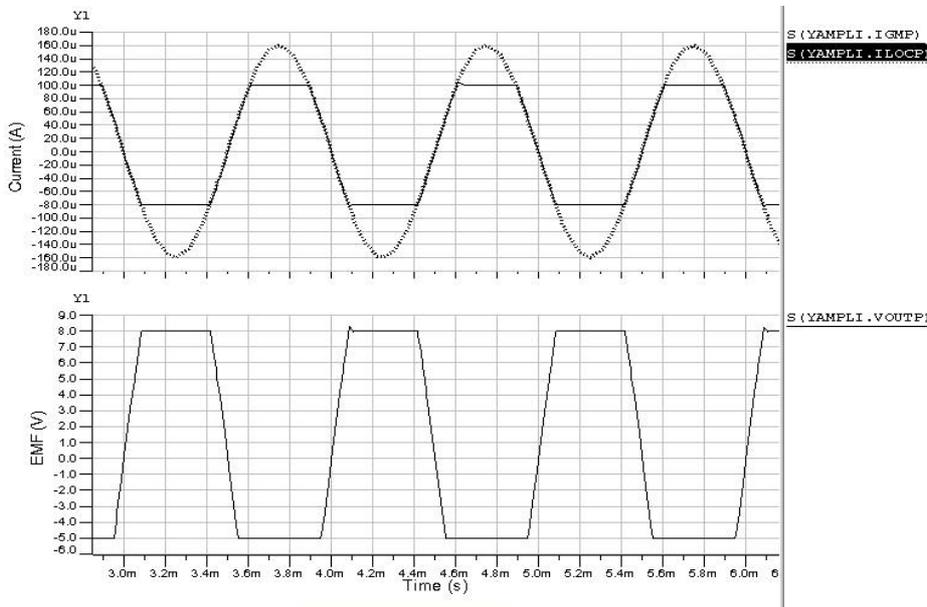
Figure 5.8:  $I_{locp}$  (dotted line),  $I_{gmp}$  (solid line) currents [A] (up) and  $V_{outp}$  [V] (down) for a time-domain simulation of the OTA model loaded by a 10 pF capacitor and driven by a fully-differential input signal with an amplitude of 0.4 V.  $g_m = 800 \mu S$ ,  $g_d = 10 \mu S$ ,  $v_{dd} = 10 V$ ,  $v_{ss} = -5 V$ ,  $i_{max} = 100 \mu A$  and  $i_{min} = -80 \mu A$ .
