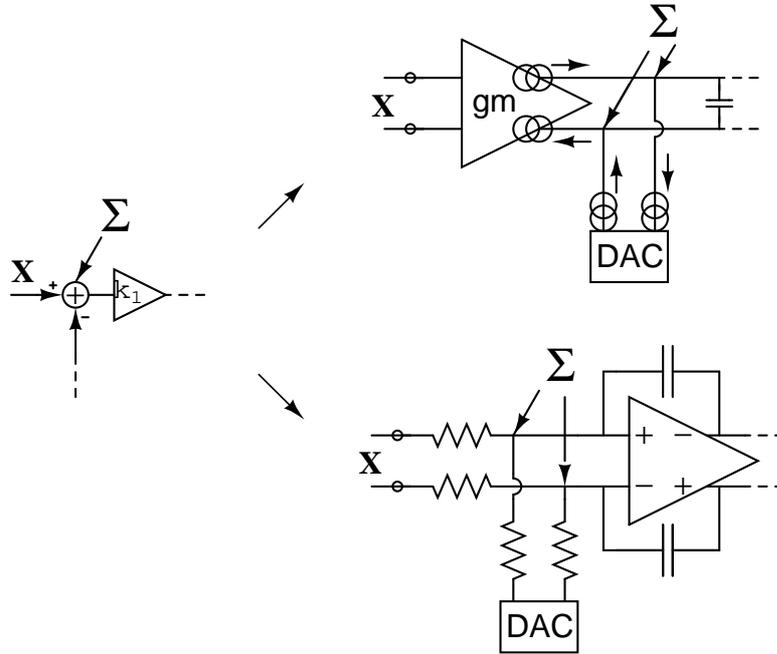
Figure 6.17: Position in the loop of the amplifier of the first integrator in the case of a  $gm-C$  type (up) and active  $RC$  (down) implementation of the integrators.  $\Sigma$  refers to the summing point as represented in the  $\Delta\Sigma$  loop schematics of Fig. 6.9 or Fig. 6.10
