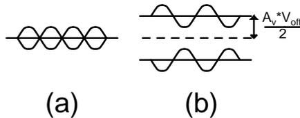
Figure 5.10: Output voltage waveforms of a fully-differential amplifier with (a) zero input-referred offset voltage ( $V_{off}$ ) and (b) non-zero  $V_{off}$ .  $A_v$  is the voltage gain of the amplifier.
