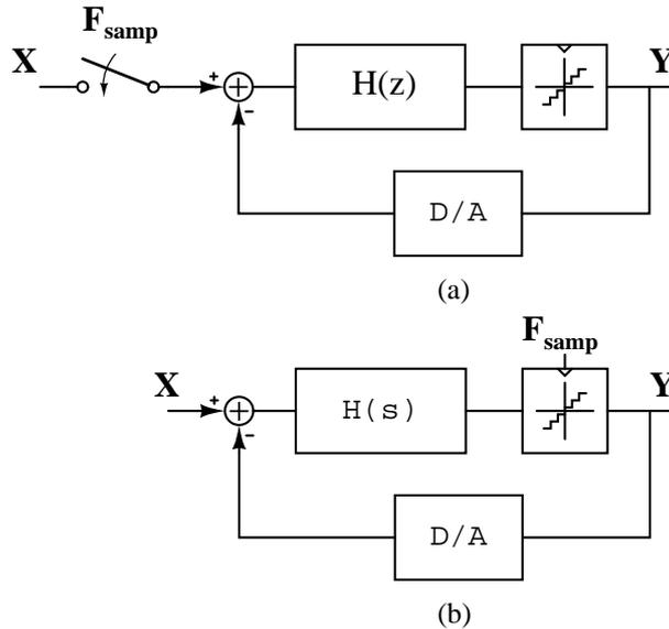
Figure 6.4: A discrete-time (DT) (a) and a continuous-time (CT)  $\Delta\Sigma$  modulator. For simplicity, only the first place where sampling occurs is indicated. The DAC's (for both DT and CT), the DT loop filter and the internal ADC (DT) are also triggered by the sampling frequency  $F_{smp}$
