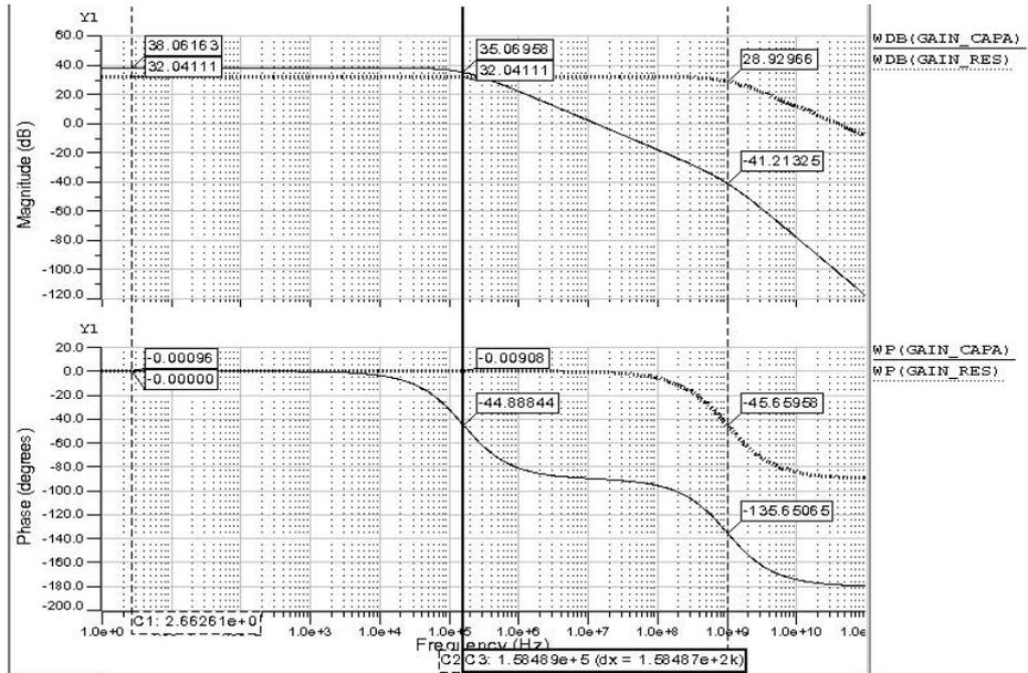
Figure 5.7: AC frequency responses in magnitude [dB] (up) and phase [°] (down) vs. frequency [Hz] for an amplifier emulated by our model. The OTA parameters are  $g_m = 800 \mu S$ ,  $g_d = 10 \mu S$  and  $f_{p\_int} = 1 GHz$ . the OTA is simulated in two cases: 1) with a 10 pF capacitive load (solid lines) and 2) with a 100 kΩ resistance (dotted lines).
