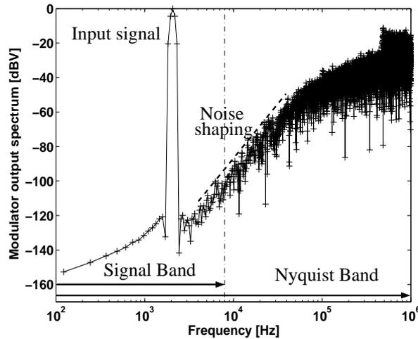
Figure 6.3: Spectrum of the modulator output [dBV] vs. frequency [Hz] for a single-bit 3rd order modulator, with  $OSR = 128$  and  $F_{samp} = 2$  MHz. A signal at 2.075 kHz is applied at the modulator input.
