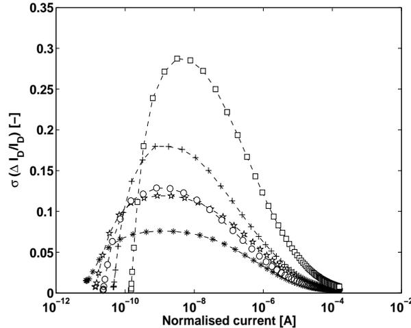
**Figure 4.1:** Measured  $\sigma(\Delta I_D/I_D)$  vs. normalized drain current ( $I_{norm}$ ) for n-type MOSFETs of a  $0.35 \mu\text{m}$  bulk CMOS technology for devices with minimal length ( $L = 0.35 \mu\text{m}$ ) and different device widths:  $W = 40 \mu\text{m}$  (\*),  $W = 20 \mu\text{m}$  (\*),  $W = 10 \mu\text{m}$  (o),  $W = 5 \mu\text{m}$  (+) and  $W = 2 \mu\text{m}$  ( $\square$ ).  $V_D = 1.3 \text{ V}$ ,  $V_S = 0 \text{ V}$ .
