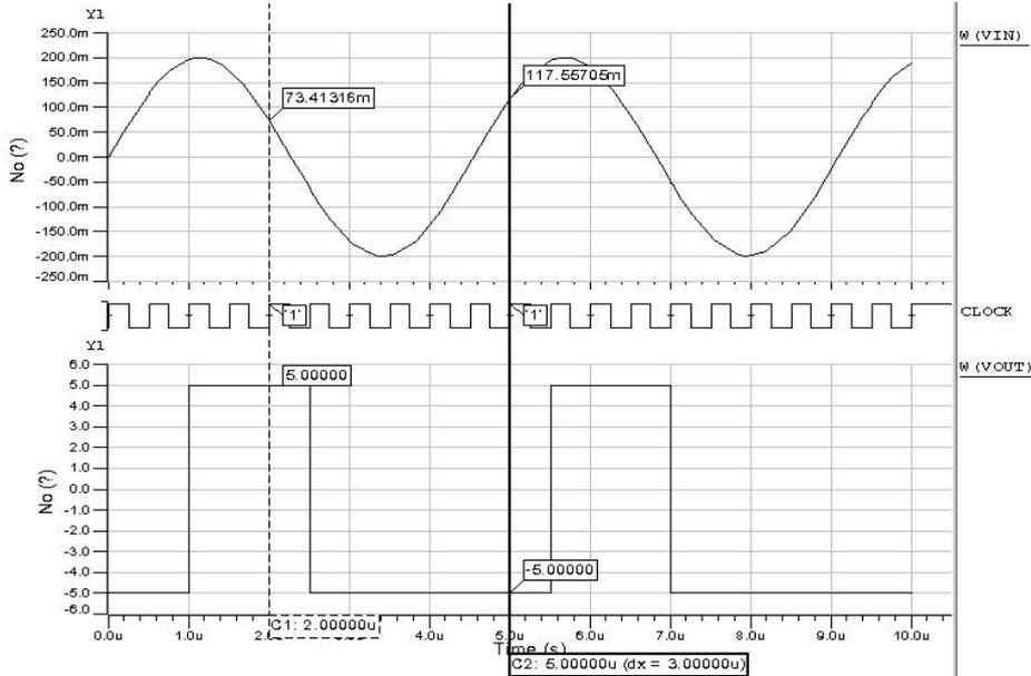
**Figure 5.20:** Architecture *comp1bitFD\_behav2* fully-differential output ( $w(vout) \equiv Voutp - Voutm[V]$ ) when driven by a fully-differential sine wave ( $w(vin) \equiv Vinp - Vmnm[V]$ ) where  $Voutp$  ( $Voutm$ ) and  $Vinp$  ( $Vmnm$ ) are the positive and negative outputs and inputs, respectively.  $offset = 100\text{ mV}$ ,  $hyst = 100\text{ mV}$ ,  $up\_val = 2.5$  and  $down\_val = -2.5$ . clock is the triggering clock.
