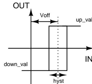
Figure 5.18: Generics associated to the VHDL-AMS entity emulating a comparator.
