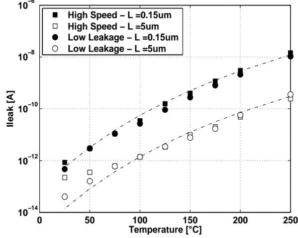
**Figure A.3: Measured  $I_{leak}$  [A] vs. temperature for n-type high speed ( $\square$ ) and low leakage ( $\circ$ ) MOSFETs. The dotted lines show the proportionality to  $n_i$ .  $I_{leak}$  is measured for  $V_G$  such that we are in the plateau region.  $L = L_{nom} = 0.15 \mu\text{m}$  (full symbols) and  $L = 5 \mu\text{m}$  (void symbols).  $W = 10 \mu\text{m}$ ,  $V_D = 1 \text{ V}$  and  $V_S = 0 \text{ V}$ .**
