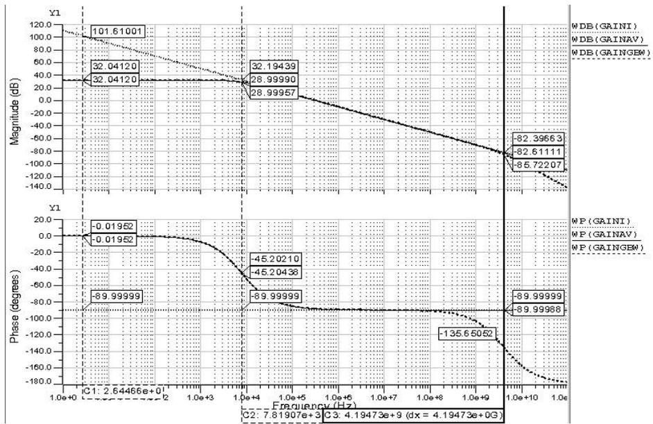
**Figure 5.22:** Magnitude [dB] (up) and phase [°] (down) for *GAINI*, *GAINAV* and *GAINBW*.  $GAINI \equiv \frac{V_{outp} - V_{outm}}{V_{inp} - V_{inm}}$  for the ideal integrator, *GAINAV* and *GAINBW* are defined in the same way but for the amplifier with finite gain and bandwidth, respectively.  $gain\_int = 2.0e6$ ,  $gain\_ampli = 40$  and  $fp\_ampli = 100.0e6$ .
