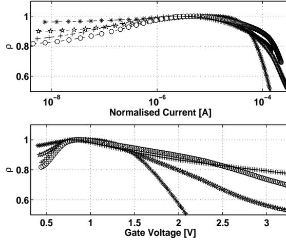
**Figure 4.3:** Correlation coefficient  $\rho$  [-] extracted from measurements vs.  $Inorm$  [A] (up) and  $V_G$  [V] (down) for n-type MOSFETs of a 0.35  $\mu\text{m}$  bulk CMOS technology for different device sizes:  $W = 40 \mu\text{m}$  and  $L = 10 \mu\text{m}$  (\*);  $W = 10 \mu\text{m}$  and  $L = 2 \mu\text{m}$  (\*);  $W = 5 \mu\text{m}$  and  $L = 0.8 \mu\text{m}$  (o);  $W = 2 \mu\text{m}$  and  $L = 0.35 \mu\text{m}$  (+).  $V_D = 1.3 \text{ V}$ ,  $V_S = 0 \text{ V}$ .
