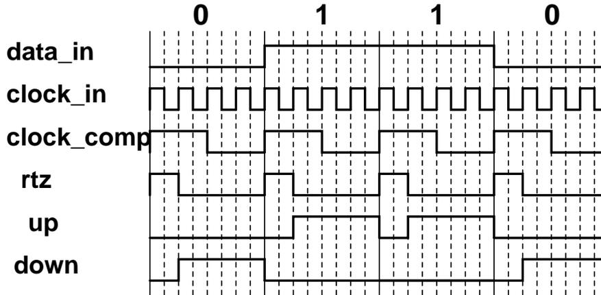
**Figure 6.31:** Time-diagram of the DAC control signals corresponding to a '0110' *data\_in* sequence. *clock\_in* is the input clock at  $4 \times F_{\text{samp}}$ . *rtz*, *up* and *down* are the three DAC control signals. *clock\_comp* oscillates at  $F_{\text{samp}}$  in order to trigger the comparator.
