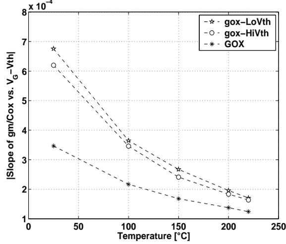
Figure 3.5: Magnitude of the decreasing slope of the  $gm/C_{ox}$  vs.  $V_G - V_{th}$  characteristic beyond its peak, in function of the temperature for gox-LoVth, gox-HiVth and GOX devices.  $W = 10 \mu m$  and  $L = 10 \mu m$  for all devices.
