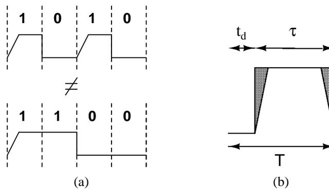
Figure 6.13: DAC waveform imperfections: (a) unequal rise and fall times of a non-return-to-zero pulse generate ISI and (b) finite settling time reduces the energy transmitted to the loop filter by the DAC.
