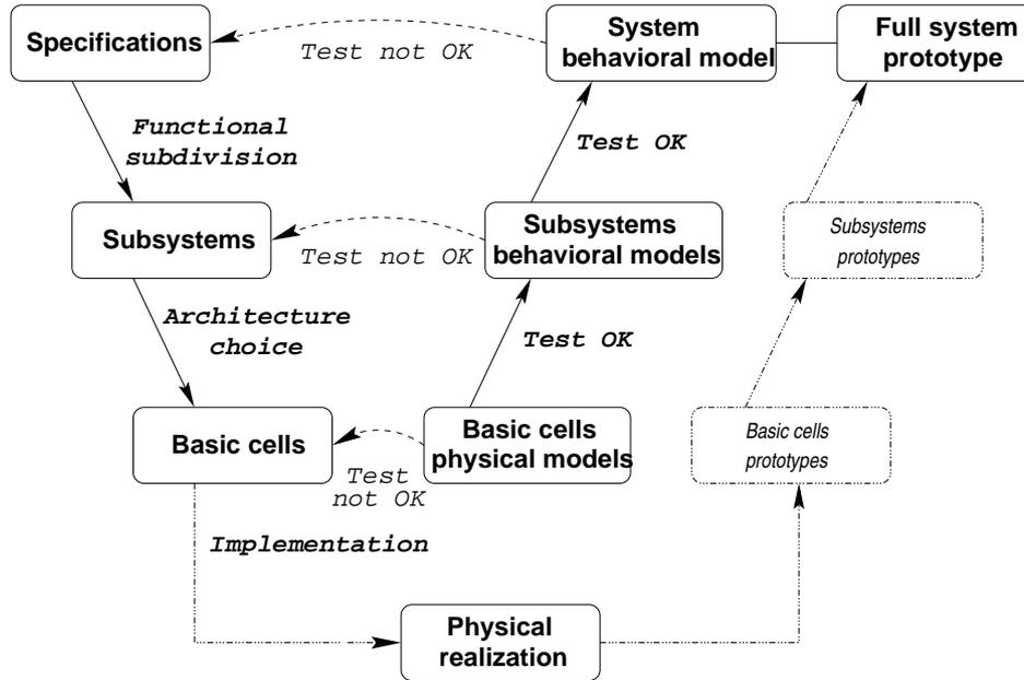
Figure 7.3: Improved top-down design and bottom-up validation design flows of analog circuits using HDL-AMS with less prototype realizations and enhanced reliability. Dotted lines indicate prototypes that could be avoided using HDL-AMS. The V-cycle of Fig. 7.1 is modified and it is called the *Virtual Prototyping Cycle* in the case all the intermediate prototypes are avoided [7].
