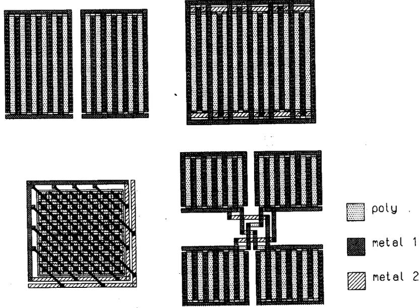
Figure C.9: Different possible layouts for the same differential pair [5].
