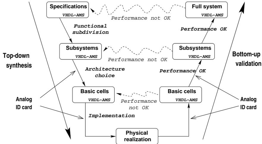
Figure 1.4: Top-down design and bottom-up validation design flows of analog circuits. VHDL-AMS provides a common description of the different abstraction levels and the analog ID card enables the transmission of relevant information: specifications and analog performance, from the basic cell level to the actual implementation and vice-versa.
