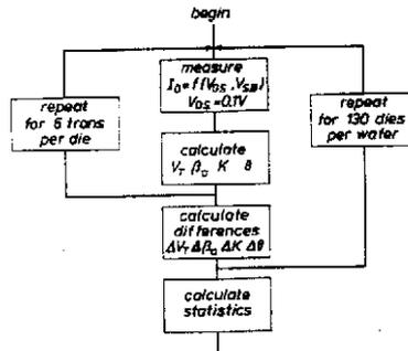
Figure C.3: Measurement procedure used by Pelgrom[6]
