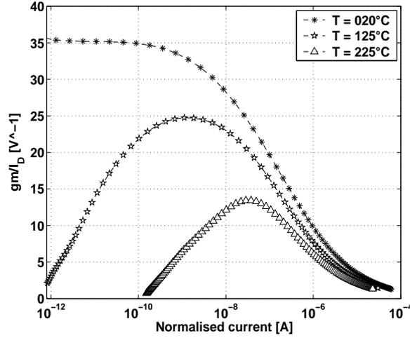
Figure 4.6: Measured  $\frac{gm}{I_D}$  [ $V^{-1}$ ] vs.  $I_{norm}$  [A] for n-type MOSFETs of a  $2\ \mu m$  fully-depleted SOI CMOS technology with  $W = 20\ \mu m$  and  $L = 10\ \mu m$  for different temperatures:  $T = 25^\circ C$  (\*),  $T = 125^\circ C$  (★) and  $T = 225^\circ C$  ( $\Delta$ ).  $V_D = 1.5\ V$ ,  $V_S = 0\ V$ .
