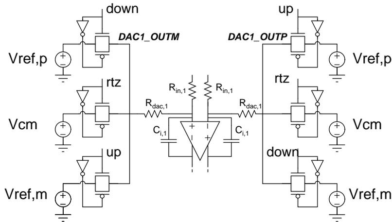
**Figure 6.30:** Architecture of the fully-differential DAC, whose outputs ( $V_{dac,outp}$  and  $V_{dac,outm}$ ) are connected to the first amplifier input through resistances  $R_{dac,1}$ .  $V_{ref,p}$  ( $V_{ref,m}$ ) is the DAC output high (low) level value and  $V_{ref,cm}$  is the common-mode value to which the outputs are connected during the return to zero. *rtz*, *up* and *down* are the clock signals and are generated by a logic circuit.
