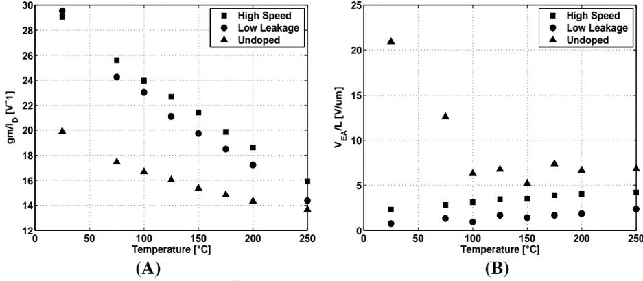
Figure 2.14: Measured  $\frac{gm}{ID}$  (A) and  $\frac{V_{EA}}{L}$  (B) vs. temperature for n-type high speed (■), low leakage (●) and undoped (▲) MOSFETs.  $\frac{gm}{ID}$  and  $V_{EA}$  are extracted for a normalized drain current  $Inorm$  corresponding to the  $\frac{gm}{ID}, max$  at 250°C.  $W = 10 \mu m$  and  $L = L_{nom} = 0.15 \mu m$  for high speed and low leakage devices.  $W = 5 \mu m$  and  $L = 0.16 \mu m$  for undoped MOSFETs.  $V_D = 1 V$  and  $V_S = 0 V$  for all.
