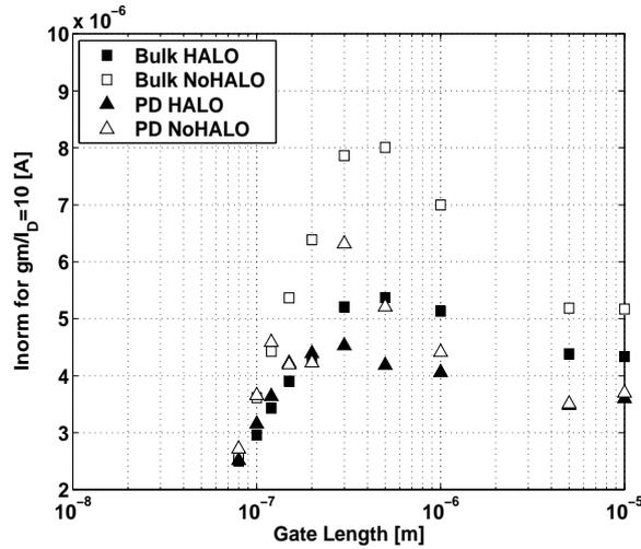
Figure 2.11: Measured  $Inorm$  corresponding to  $\frac{gm}{I_D} = 10 [V^{-1}]$  vs. gate length for n-type MOSFETs: Bulk ( $\square$ ) and PD SOI ( $\triangle$ ) with (full symbols) and without HALO implantation (void symbols).  $W = 10 \mu m$  for all devices,  $L_{nom} = 0.12 \mu m$ ,  $V_D = 0.75 V$  and  $V_S = 0 V$ .
