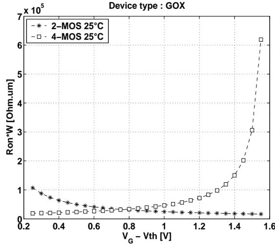
Figure 3.9:  $R_{on} * W$  [ $\Omega \cdot \mu m$ ] vs.  $V_G - V_{th}$  for 2-MOS and 4-MOS resistive structures with GOX devices at 25°C.  $V_{G, fixed} = 2 V$  and  $L = 10 \mu m$ .
