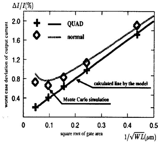
Figure C.10: The layout type has an impact on the performance of a current mirror [2]
