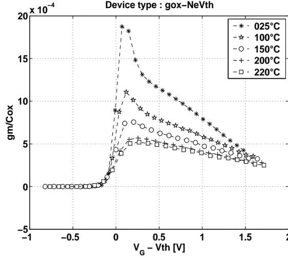
**Figure 3.6:**  $g_m$  [A/V] vs.  $V_G - V_{th}$  for gox-NeVth (thin-gate oxide, natural doping) device,  $L = 20 \mu m$ ,  $W = 20 \mu m$  and  $V_d = 50 mV$ .
