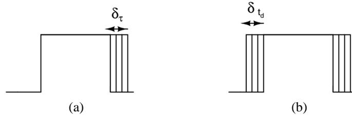
Figure 6.14: Different jitter mechanisms in a return-to-zero DAC pulse: (a) pulse width jitter (constant  $t_d$ ) and (b) pulse delay jitter (constant  $\tau$ ).
