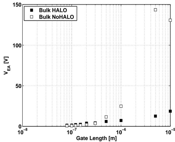
Figure 2.9: Measured  $V_{EA}$  at  $I_{norm} = 4 \mu A$  vs. gate length for n-type Bulk MOSFETs, with (full symbols) and without HALO implantation (void symbols).  $W = 10 \mu m$ ,  $L_{nom} = 0.12 \mu m$ ,  $V_D = 0.75 V$  and  $V_S = 0 V$ .
