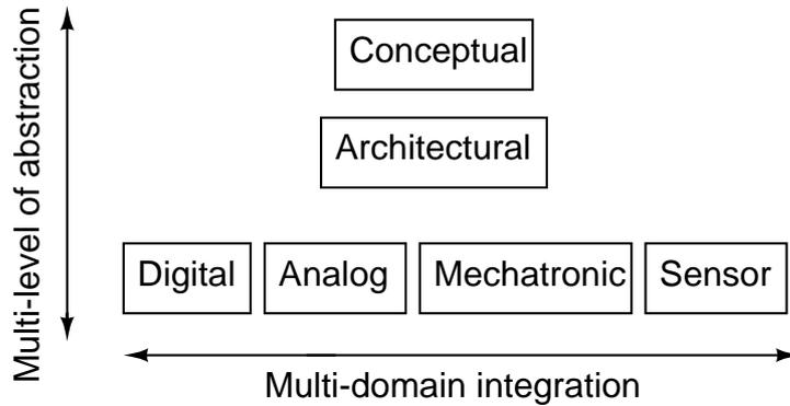
Figure 5.3: VHDL-AMS is a true multi-abstraction, multi-domain description and simulation tool
