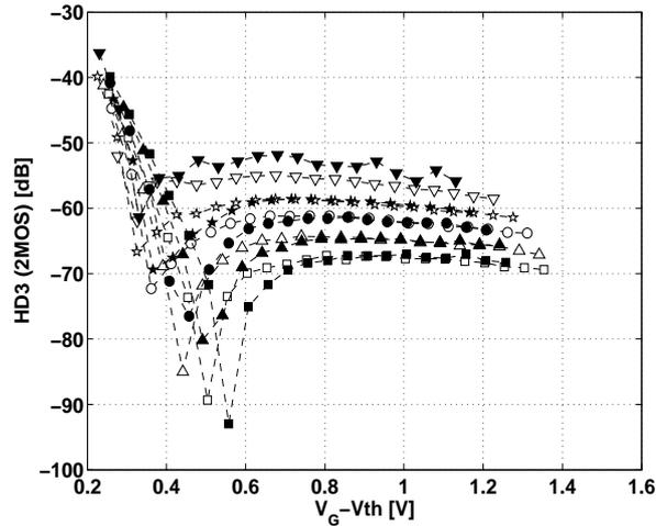
Figure 3.7: HD3[dB] vs.  $V_G - V_{th}$  for 2-MOS resistive structures with gox-LoVth (thin-gate oxide, low  $V_{th}$ ) (void symbols) and gox-HiVth (thin-gate oxide, high  $V_{th}$ ) (full symbols),  $W = L = 10 \mu m$  at different temperatures: 25°C ( $\nabla$ ), 100°C ( $*$ ), 150°C ( $\circ$ ), 200°C ( $\Delta$ ) and 220°C ( $\square$ )
