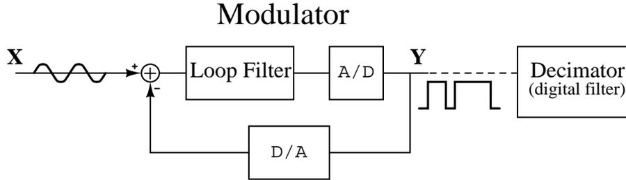
**Figure 5.1:** A  $\Delta\Sigma$  analog-to-digital converter is the series combination of a mixed-signal modulator and a digital filter, the decimator. The modulator is composed of an analog loop filter, an internal analog-to-digital converter and a feedback digital-to-analog converter.
