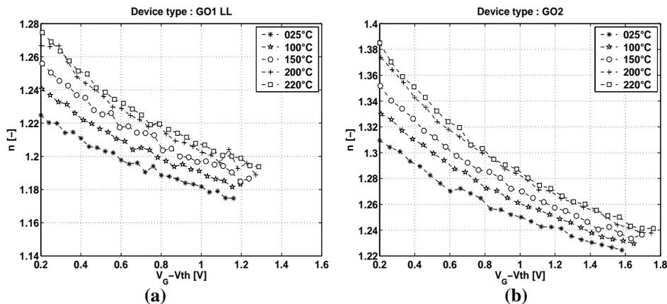
Figure B.1:  $n$  body effect factor in strong inversion [-] vs.  $V_G - V_{th}$  for (a) GO1 LL device (thin-gate oxide, high  $V_{th}$ ) and (b) GO2 (thick-gate oxide) device at different temperatures.  $W = 10 \mu m$  and  $L = 10 \mu m$ .
