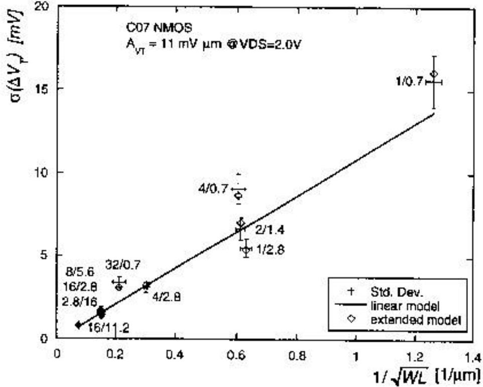
Figure C.4: Threshold voltage mismatch for NMOS transistors in saturation [5]
