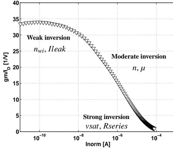
Figure 2.3: Typical  $\frac{gm}{I_D}$  ratio vs.  $Inorm$  showing the different regions of inversion and the main physical parameters playing a role in weak ( $n_{wi}$ , the inverse of the subthreshold slope and  $I_{leak}$ , the leakage current), in moderate ( $n$ , the linearized body effect factor and  $\mu$  the mobility) and strong inversion ( $vsat$ , the velocity saturation and  $R_{series}$ , the series resistance).
