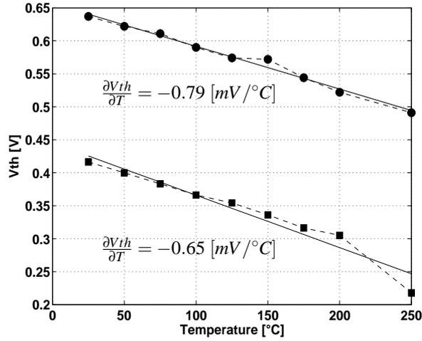
**Figure A.4:** Measured  $V_{th}$  [V] vs. temperature for n-type high speed (■) and low leakage (●) MOSFETs.  $W = 10 \mu\text{m}$  and  $L = L_{nom} = 0.15 \mu\text{m}$ .  $V_D = 50 \text{ mV}$  and  $V_S = 0 \text{ V}$ .
