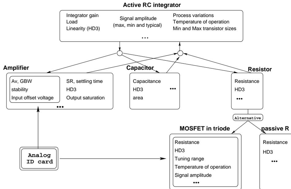
Figure 7.8: Top-down propagation of the specifications and bottom-up characterization in the case of an active RC integrator. The contribution of the analog ID card is highlighted.
