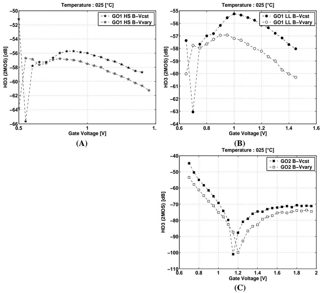
Figure B.2: HD3[dB] vs.  $V_G$  for 2-MOS structures composed of devices GO1 HS (thin-gate oxide, low  $V_{th}$ )(A), GO1 LL (thin-gate oxide, high  $V_{th}$ )(B) and GO2 (thick-gate oxide) (C) with body connected to the fixed potential terminal (full symbols) and with body connected to the varying signal source (void symbols). All devices are  $10 \mu\text{m}$  long and  $10 \mu\text{m}$  large.  $V_a = 200 \text{ mV}$  around  $V_o = 0 \text{ V}$ , at room temperature.
