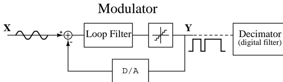
**Figure 6.1:** A  $\Delta\Sigma$  analog-to-digital converter is the series combination of a mixed-signal modulator and of a digital filter, the decimator. The modulator is composed of an analog loop filter, an internal analog-to-digital converter and a feedback digital-to-analog converter.
