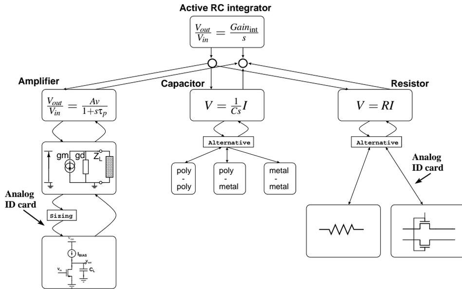
Figure 7.7: Top-down structural division of an active RC integrator starting from the system behavioral description down to the physical realization for the three subsystems: amplifier, resistance and capacitance. The interaction of the analog ID card is highlighted.
