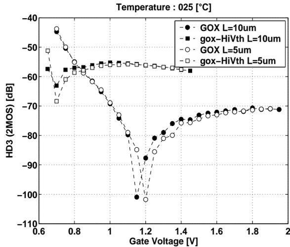
Figure 3.10: HD3[dB] vs.  $V_G$  at room temperature for 2-MOS resistive structures with gox-HiVth (thin-gate oxide, high  $V_{th}$ ) ( $\square$ ) and with GOX (thick-gate oxide) ( $\circ$ ).  $L = 5 \mu\text{m}$  (void symbols) and  $L = 10 \mu\text{m}$  (full symbols).
