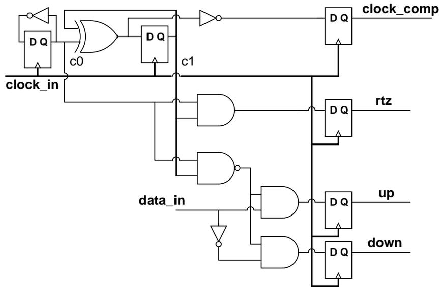
Figure 6.32: DAC RTZ logic. *clock\_in* is the input clock at  $4 \times F_{\text{samp}}$  and *data\_in* is the comparator output data. *rtz*, *up* and *down* are the three DAC control signals. *clock\_comp* oscillates at  $F_{\text{samp}}$  in order to trigger the comparator
