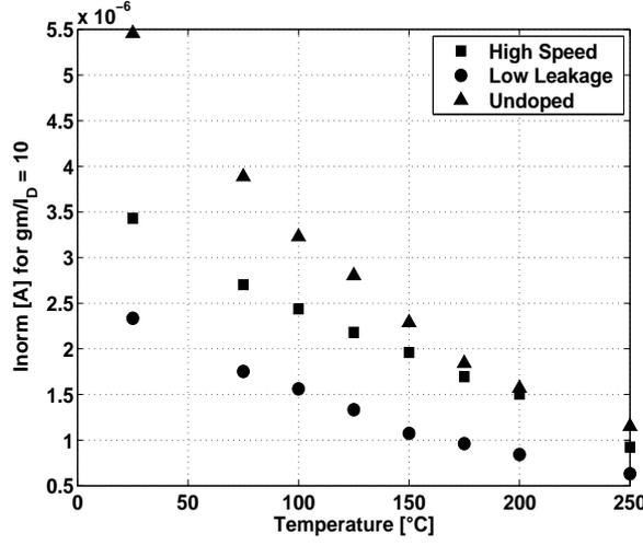
Figure 2.13: Measured  $Inorm$  [A] corresponding to a  $\frac{gm}{ID} = 10$  [ $V^{-1}$ ] vs. temperature for n-type high speed (■), low leakage (●) and undoped (▲) MOSFETs.  $W = 10 \mu m$  and  $L = L_{nom} = 0.15 \mu m$  for high speed and low leakage devices.  $W = 5 \mu m$  and  $L = 0.16 \mu m$  for undoped MOSFETs.  $V_D = 1 V$  and  $V_S = 0 V$  for all.
