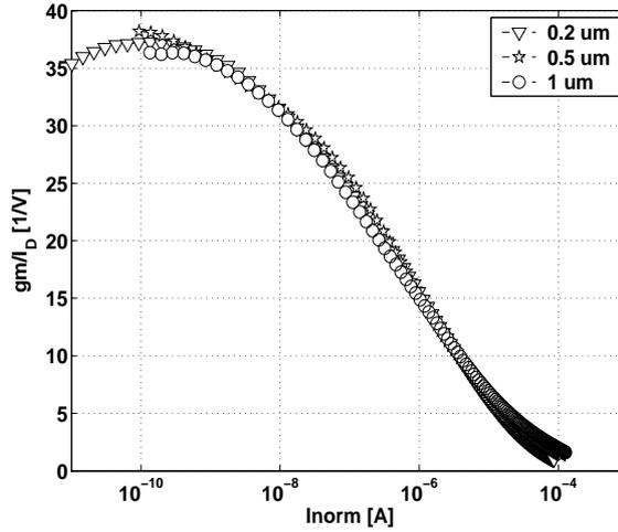
**Figure 2.2:** Measured  $\frac{gm}{I_D}$  ratio vs.  $Inorm$  for n-type MOSFETs of a fully-depleted silicon-on-insulator 0.15  $\mu m$  technology with  $L = 0.2 \mu m$  ( $\nabla$ ),  $L = 0.5 \mu m$  ( $*$ ),  $L = 1 \mu m$  ( $\circ$ ).  $W = 10 \mu m$  for all devices,  $V_D = 0.75 V$ ,  $V_S = 0 V$ .
