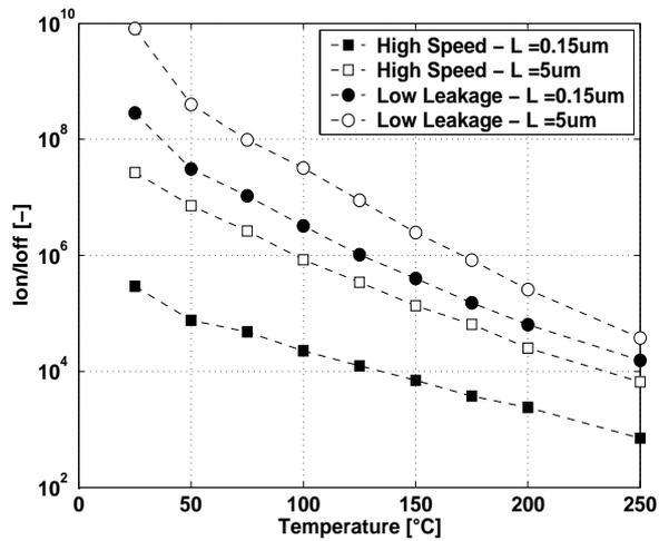
Figure A.2: Measured  $I_{on}/I_{off}$  ratio vs. temperature for n-type high speed ( $\square$ ) and low leakage ( $\circ$ ) MOSFETs.  $I_{on}$  is measured for  $V_G = 1.5\text{ V}$ ,  $I_{off}$  for  $V_G = 0\text{ V}$ .  $L = L_{nom} = 0.15\ \mu\text{m}$  (full symbols) and  $L = 5\ \mu\text{m}$  (void symbols).  $W = 10\ \mu\text{m}$ ,  $V_D = 1\text{ V}$  and  $V_S = 0\text{ V}$ .
