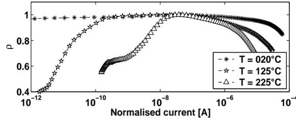
Figure 4.7: Correlation coefficient  $\rho$  [-] extracted from measurements vs.  $I_{norm}$  [A] for n-type MOSFETs of a  $2\ \mu m$  fully-depleted SOI CMOS technology with  $W = 20\ \mu m$  and  $L = 10\ \mu m$  for different temperatures:  $T = 25^\circ C$  (\*),  $T = 125^\circ C$  (★) and  $T = 225^\circ C$  ( $\Delta$ ).  $V_D = 1.5\ V$ ,  $V_S = 0\ V$ .
