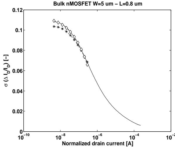
**Figure 4.8:**  $\sigma_{(\Delta I_D/I_D)}$  [-] vs.  $I_{norm}$  [A] for a n-type MOSFET of the  $0.35 \mu m$  bulk CMOS technology with  $W = 5 \mu m$  and  $L = 0.8 \mu m$ . The solid line is the measured  $\sigma_{(\Delta I_D/I_D)}$  for  $V_D = 1.5 V$ ,  $V_S = 0 V$ . In weak and moderate inversion, ( $\diamond$ ) is our proposed new term:  $f(V_G)\Delta n$  and (\*) is the classical assumption:  $\frac{gm}{I_D}\Delta V_{th}$ .
