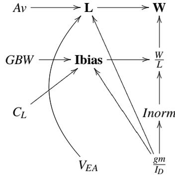
Figure 2.4: Top-down  $\frac{gm}{I_D}$  design methodology of a common-source amplifier. The design specifications are  $Av$ ,  $GBW$  and  $C_L$  while the transistor performance is described by the  $\frac{gm}{I_D}$  vs.  $Inorm$  characteristic and  $V_{EA}$ . The results are  $W$ ,  $L$  and  $I_{bias}$ .
