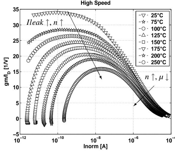
**Figure 2.12:** Measured  $\frac{gm}{I_D}$  [ $V^{-1}$ ] vs.  $Inorm$  [A] characteristic for a n-type high speed (low  $V_{th}$ ) MOSFET as a function of the temperature from room temperature up to 250°C.  $W = 10 \mu m$ ,  $L = L_{nom} = 0.15 \mu m$ ,  $V_D = 1 V$  and  $V_S = 0 V$ .
