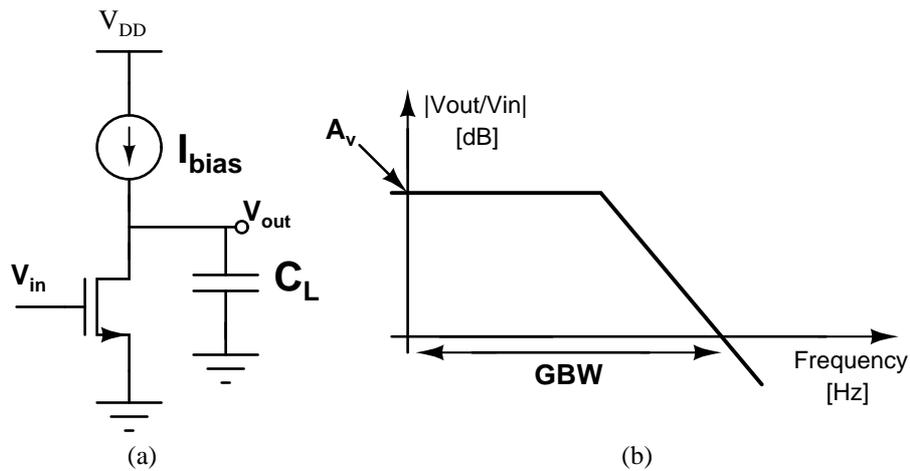
**Figure 2.1:** (a) Common-source amplifier stage: MOSFET transistor biased by a DC current source ( $I_{bias}$ ) and loaded by a capacitance ( $C_L$ ). (b) Major analog characteristics of an amplifier: low-frequency gain ( $A_v$ ) and gain-bandwidth product ( $GBW$ ).
