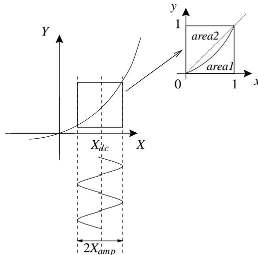
Figure D.1: The zone of interest of the *Y* vs. *X* characteristic is normalized in the first quadrant into a *y* vs. *x* characteristic.
