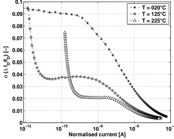
**Figure 4.5:** Measured  $\sigma_{(\Delta I_D/I_D)}$  [-] vs.  $I_{norm}$  [A] for n-type MOSFETs of a 2  $\mu\text{m}$  fully-depleted SOI CMOS technology with  $W = 20 \mu\text{m}$  and  $L = 10 \mu\text{m}$  for different temperatures:  $T = 25^\circ\text{C}$  (\*),  $T = 125^\circ\text{C}$  (★) and  $T = 225^\circ\text{C}$  ( $\Delta$ ).  $V_D = 1.5 \text{ V}$ ,  $V_S = 0 \text{ V}$ .
