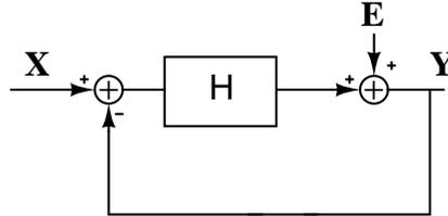
Figure 6.2: Linear model of a  $\Delta\Sigma$  modulator, in which the 1-bit internal quantizer is modeled by an additive noise source.  $H$  is the loop filter transfer function.
