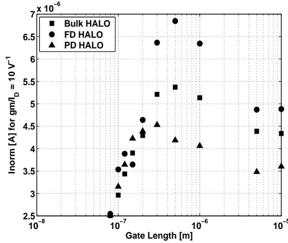
**Figure 2.10:** Measured  $Inorm$  corresponding to  $\frac{gm}{I_D} = 10 \text{ [V}^{-1}\text{]}$  vs. gate length for n-type MOSFETs: Bulk ( $\square$ ), FD SOI ( $\circ$ ) and PD SOI ( $\Delta$ ) with HALO implantation.  $W = 10 \text{ }\mu\text{m}$  for all devices,  $L_{nom} = 0.12 \text{ }\mu\text{m}$ ,  $V_D = 0.75 \text{ V}$  and  $V_S = 0 \text{ V}$ .
