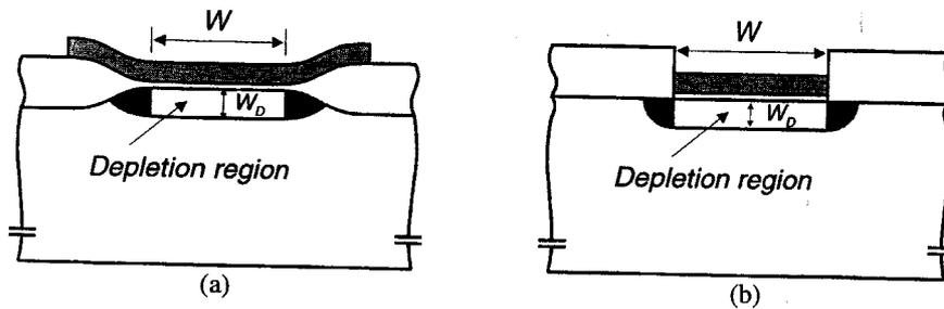
Figure C.6: Depletion region depth when transistor width is small. Real situation (a) and approximation (b) [5]
