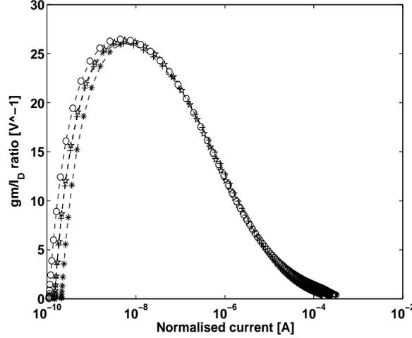
Figure 4.4: Measured  $\frac{gm}{I_D}$  ratio [ $V^{-1}$ ] vs.  $I_{norm}$  [A] for n-type MOSFETs of a  $0.35 \mu m$  bulk CMOS technology for different device sizes:  $W = 40 \mu m$  and  $L = 10 \mu m$  (\*);  $W = 10 \mu m$  and  $L = 2 \mu m$  (★);  $W = 5 \mu m$  and  $L = 0.8 \mu m$  (◊);  $W = 2 \mu m$  and  $L = 0.35 \mu m$  (+).  $V_D = 1.3 V$ ,  $V_S = 0 V$ .
