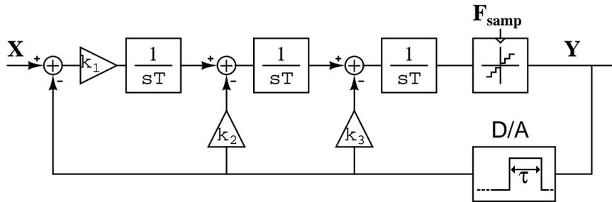
Figure 6.9: 3rd order CT  $\Delta\Sigma$  modulator stabilized by feedback.  $k_1$ ,  $k_2$  and  $k_3$  are the loop filter coefficients
