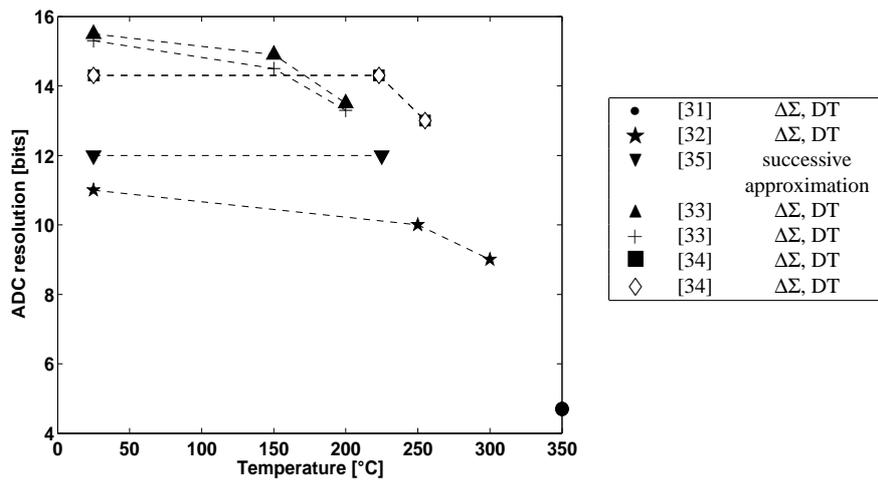
**Figure 6.6: Resolution [bits] vs. Temperature [ $^{\circ}\text{C}$ ] of the different published or commercially available ADC's targeting high temperature operation**
