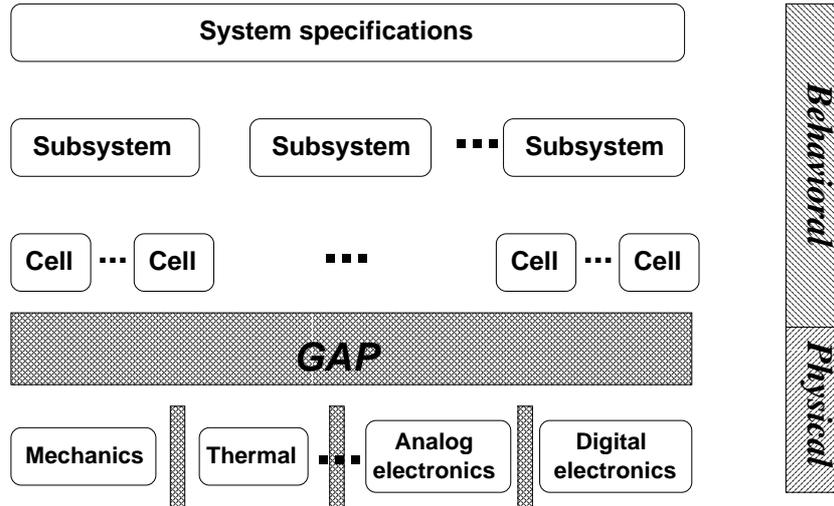
Figure 7.2: Top-down division of a multi-domain multi-signal electronic system and associated level of abstraction; from the system down to the basic cells implemented in various physical domains. Current gaps between 1) the different physical domains 2) the behavioral and physical levels of abstraction.
