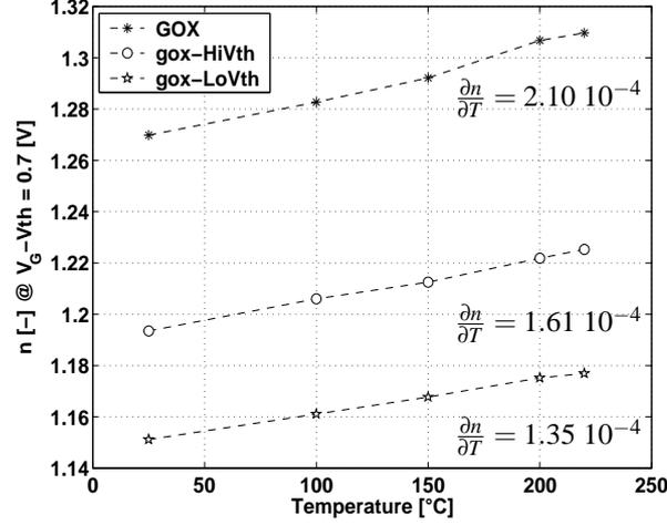
Figure 3.4:  $n$  body effect factor [-] for  $V_G - V_{th} = 0.7$  V vs. temperature for gox-LoVth, gox-HiVth and GOX devices. The slope of  $n$  vs. temperature ( $[-/^{\circ}C]$ ) is given next to the curves.  $W = 10 \mu m$  and  $L = 10 \mu m$  for all devices.
