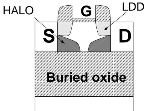
Figure 2.6: Cross-section of a silicon-on-insulator transistor showing the LDD regions and HALO doping.
