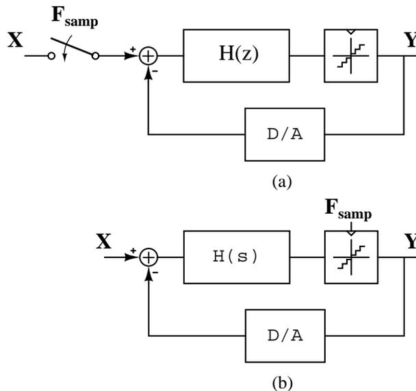
Figure 5.2: A discrete-time (DT) (a) and a continuous-time (CT) (b)  $\Delta\Sigma$  modulator. For simplicity, only the first place where sampling occurs is indicated. The DACs (for both DT and CT), the DT loop filter and the internal ADC (DT) are also triggered by the sampling frequency  $F_{smp}$
