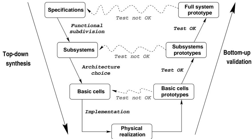
Figure 7.1: Traditional top-down design and bottom-up validation design flows of analog circuits, usually referred to as the V-cycle.
