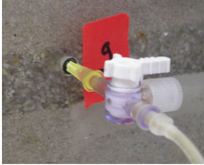
Figure C.4: Pressure measurement port. The scale is given by the size of the material 1 layer ( \approx 2 cm).
