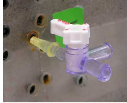
Figure C.5: Liquid phase sampling port. The scale is given by the size of the material 3 layer ( \approx 4 cm).
