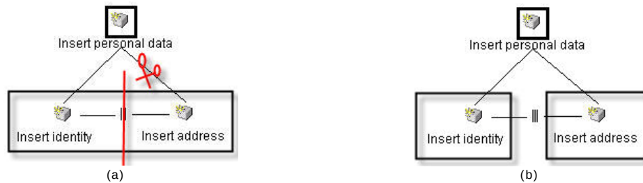
Figure 5-9 Splitting an interaction space at the level of a concurrent operator
