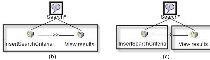
Figure 5-7 Task model for a simple IR system, with different distribution of tasks among interaction spaces
