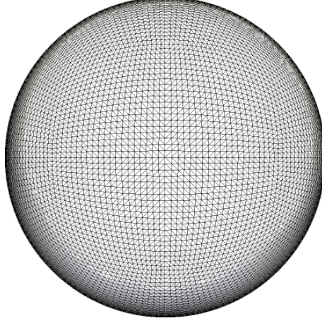
Figure 2.3: Prismatic mesh used for the OpenFOAM finite volume computation (it has been obtained as an extruded surface mesh from a cube projected onto a sphere).
