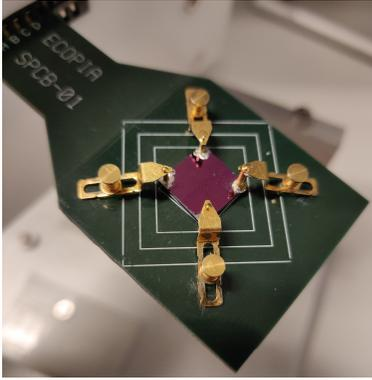
(a) PCB sample holder and electrical connections
