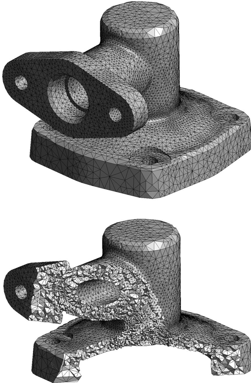
Figure III.13: Mesh adaptation based on error minimization: adapted mesh, with the initial mesh and the size field shown resp. in Figure III.12(b) and (c).
