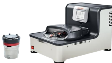
Figure 2.1 The photograph of the Planetary Micro Mill PULVERISETTE 7 (right) and EASY GTM-bowl (left).
