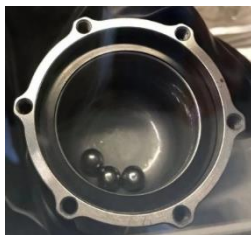
Figure 4.14 Photograph of sample used for isolating the \text{Na}[\text{AlH}(\text{CH}_3\text{NHBH}_3)_3] intermediate after 15 cycles of milling before drying.
