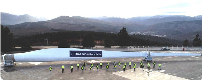
**Fig. 1.3** Thermoplastic blade manufactured as part of the ZEBRA project in 2022. Photo credit: ZEBRA consortium.
