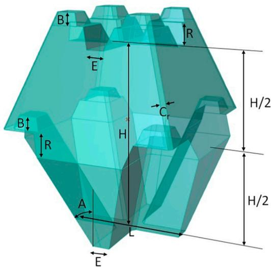
**Fig. 3.** Three-dimensional model of a droxel and definition of the parameters governing its geometry.
