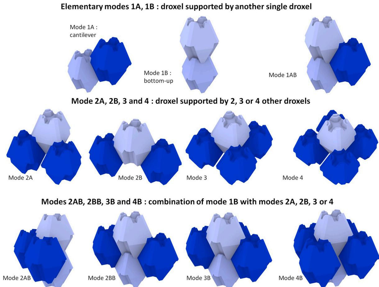
Fig. 8. Graphical description of all the possible droxels stacking modes.
