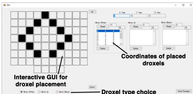
Fig. 16. Interactive GUI for the visual placement of drexels.
