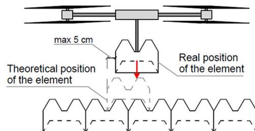
**Fig. 4.** Spatial laying tolerance allowed for the placement of UAV-compatible elements.
