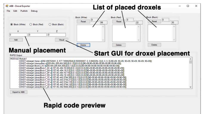
Fig. 15. Screenshot of the main window of the developed software.
