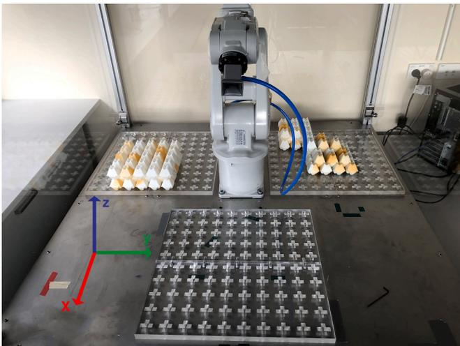
Fig. 10. ABB IRB120 robotic arm used in the experiments and positioning of the foundation plates hosting the source droxels.
