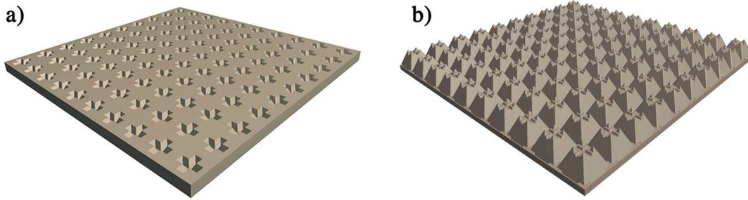
Fig. 9. Two possible arrangements for foundation pads of droxel structures: (a) “negative” foundation, (b) “positive” foundation.
