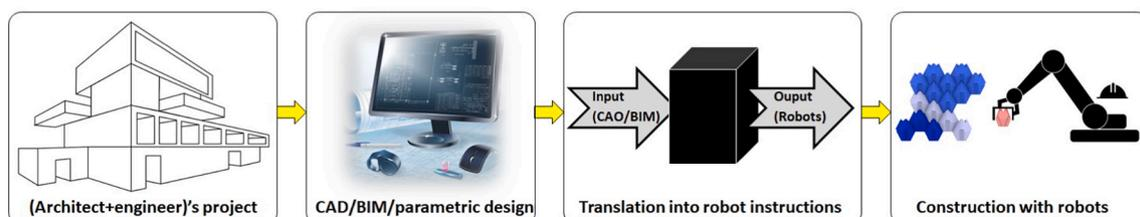
Fig. 1. Idealized workflow for the data exchange between BIM models and robotic construction components. No paper plans are produced in the process.
