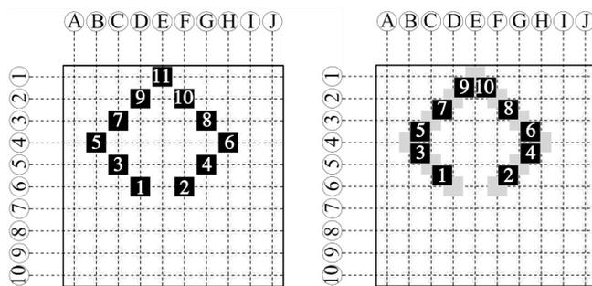
Fig. 14. First two layers of a square-based shelter construction: the order of placement of each droxel is given by the numbers reported.
