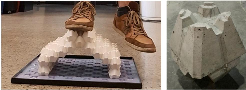
Fig. 5. On the left, small-scale tests on FDM 3D printed droxels. On the right, a 15 kg concrete droxel, under one of its possible geometrical forms.
