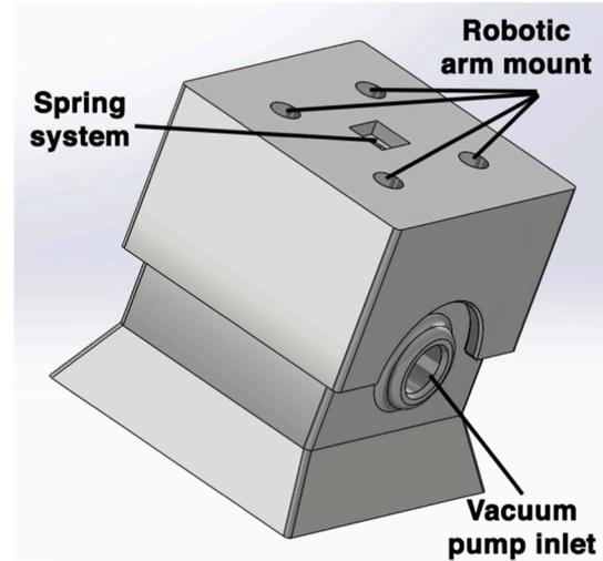
Fig. 11. The designed 3D printed end-actuator used in the experimental campaign.
