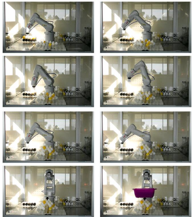
Fig. 17. Automated construction of a drexel-based shelter. From left to right, top to bottom, the placement of the 8 layers composing the structures.
