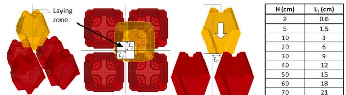
**Fig. 19.** Geometrical definition and quantitative description of the laying tolerance.
