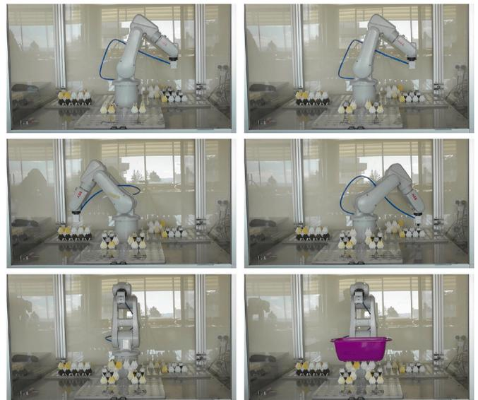
Fig. 18. Automated construction of a drexel-based bridge. From left to right, top to bottom, the placement of the 6 layers composing the structures.
