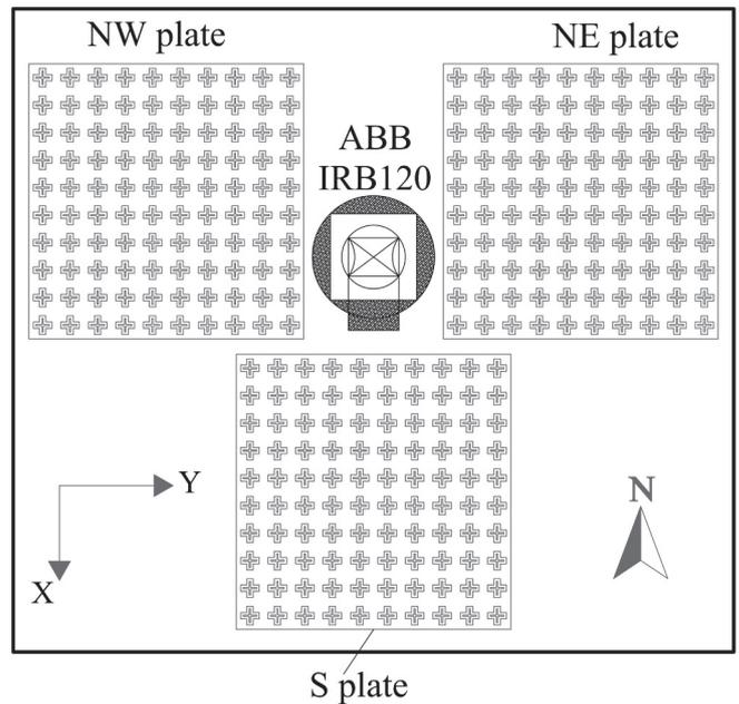
Fig. 7. Schematic representation of the controlled experimental environment. Definition of NE, NW and S foundation plates and global coordinate system.
