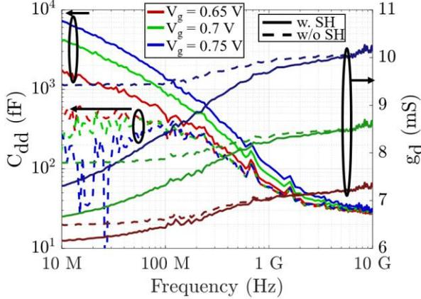
FIGURE 2, Output capacitance ( $C_{dd}$ ) and conductance ( $g_d$ ) versus frequency for different gate biases,  $V_d = 0.8$  V and  $V_{bg} = 0$  V. Measurements from which dynamic SHE is removed in dashed lines and including it in solid lines. The resonances in  $C_{dd}(f)$  below 100 MHz for  $V_g = 0.75$  V (dashed line) are due to a slightly imperfect removal of SHE resulting from a noisy subtraction of two large values.
