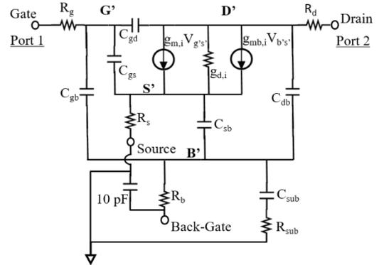
FIGURE 1. Small-signal equivalent circuit (SSEC) of an FD SOI including the back-gate and substrate nodes.
