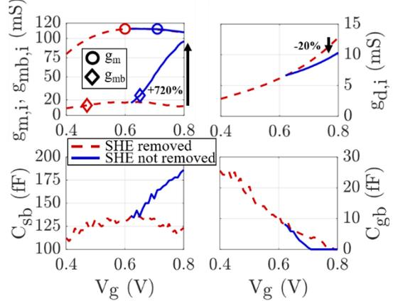
FIGURE 3.  $g_{m,i}$  and  $g_{mb,i}$  (top left),  $g_{d,i}$  (top right),  $C_{sb}$  (bottom left) and  $C_{gb}$  (bottom right) parameters of the SSEC from Fig. 1 versus  $V_g$ . Extractions based on either  $Y_{ij,iso}$  (SHE removed, in dashed lines) or  $Y_{ij}$  (SHE not removed, in solid lines) fitting from  $\sim 30$  MHz to 10 GHz.  $V_d = 0.8$  V and  $V_{bg} = 0$  V.
