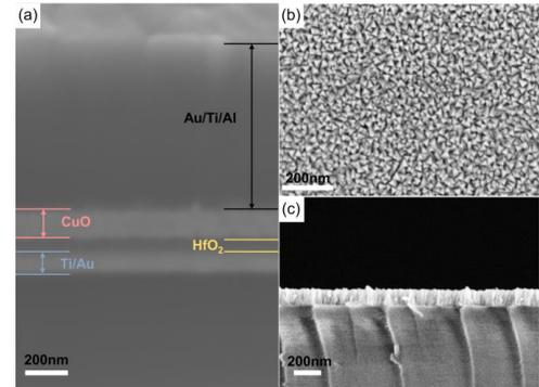
FIG.3. (a) SEM cross-section image of CuO TFT. (b) SEM plain-section and (c) SEM cross-section images of CuO thin film on SLG substrate.
