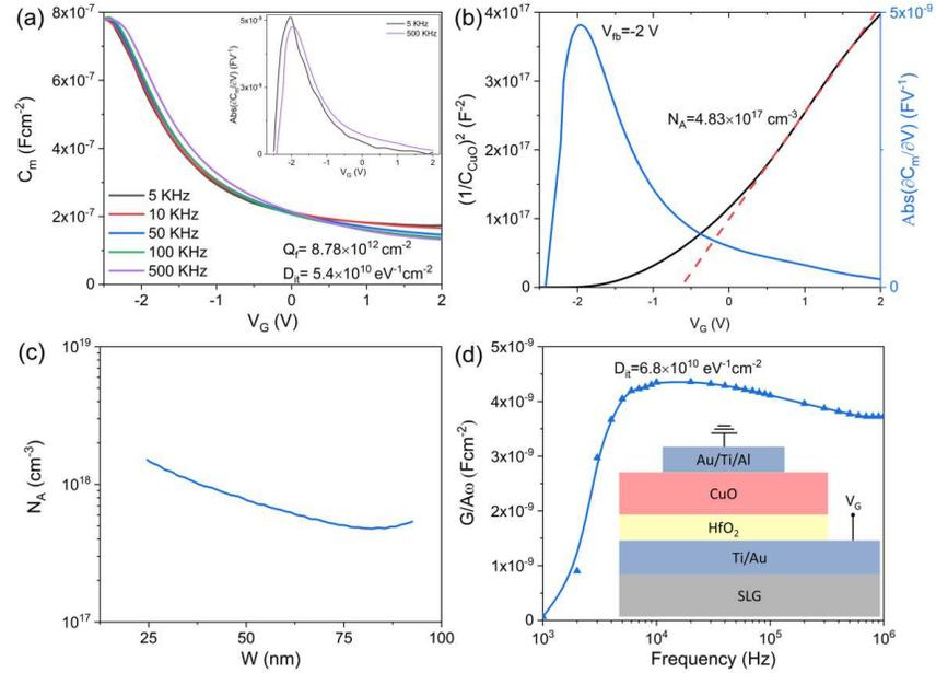
FIG. 4. (a) Corrected  $C_m$ - $V_G$  curves from 5 kHz to 500 kHz, the insets are  $abs(\partial C_m/\partial V_G)$ - $V_G$  curves at 5 and 500 kHz. (b) Calculated  $(1/C_{CuO})^2$ - $V_G$ ,  $abs(\partial C_m/\partial V_G)$ - $V_G$  and (c)  $N_A$ - $W$  curves at 500 kHz. (d)  $G/A\omega$  curve from 1 kHz to 1 MHz at 0V, the inset is the schematic of MOS capacitor.
