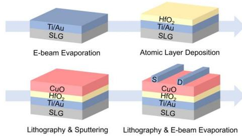
FIG. 1. Schematics for fabrication process and structure of CuO TFT.
