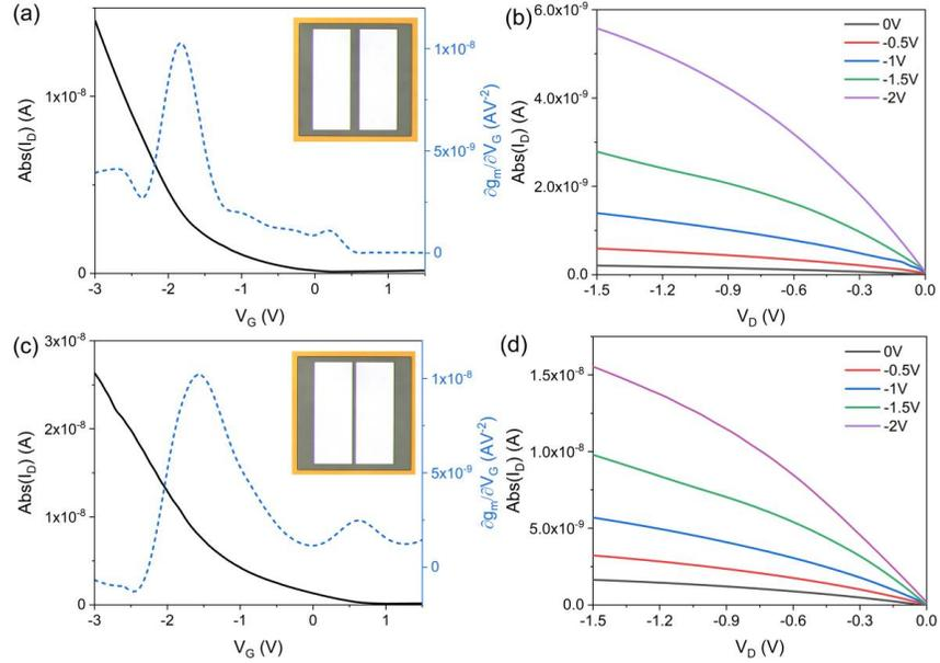
FIG. 5. Transfer  $I_D$ - $V_G$  curves ( $V_D=-1$  V) and transconductance derivatives (blue dashed lines) of CuO TFTs with channel lengths of (a) 25  $\mu\text{m}$  (c) and 10  $\mu\text{m}$  (Insets are the corresponding top-viewed photographs by optical microscope). Output  $I_D$ - $V_D$  curves ( $V_G=-2$  V to 0 V) of CuO TFTs with channel lengths of (b) 25  $\mu\text{m}$ . and (d) 10  $\mu\text{m}$ .
