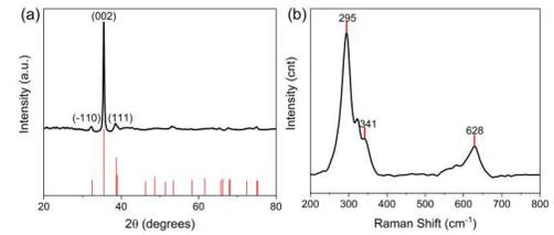
FIG. 2. (a) XRD pattern (JCPDS-45-0937) and (b) Raman spectra of deposited CuO thin film.
