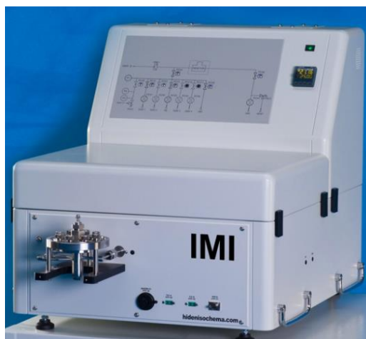
Figure 2. Adsorption device, Hidden IMI-HTP analyzer that used in this work, picture taken from: https://hidenisochema.com/hiden-products/imi-http/
