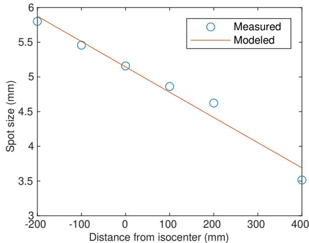
**Figure 6.** Spot sizes in  $Y$  direction at various distances from isocenter, for a proton beam of 120 MeV.
