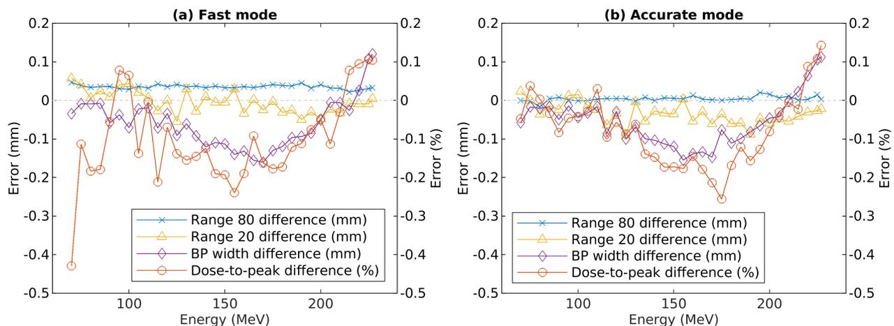
**Figure 1.** Evaluation of the accuracy of the energy spectrum tuning using (a) the fast mode; (b) the accurate mode. Error metrics are obtained after running a MCsquare simulation of a single pencil beam in water and comparing with commissioning measurements.
