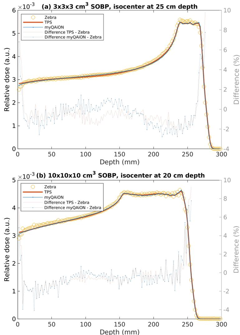
**Figure 4.** SOBPs in water: comparison of Zebra, TPS and *myQA iON* for high energy SOBPs: (a)  $3 \times 3 \times 3 \text{ cm}^3$ , (b)  $10 \times 10 \times 10 \text{ cm}^3$ .
