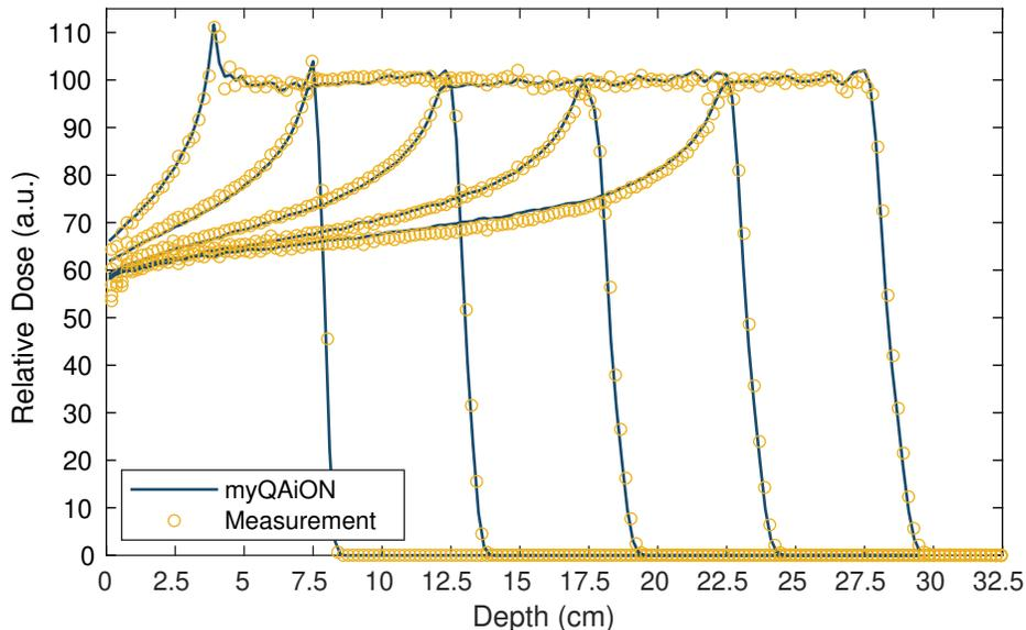
**Figure 3.** SOBPs of  $5 \times 5 \times 5 \text{ cm}^3$  in water: comparison between Zebra measurements and *myQA iON*.
