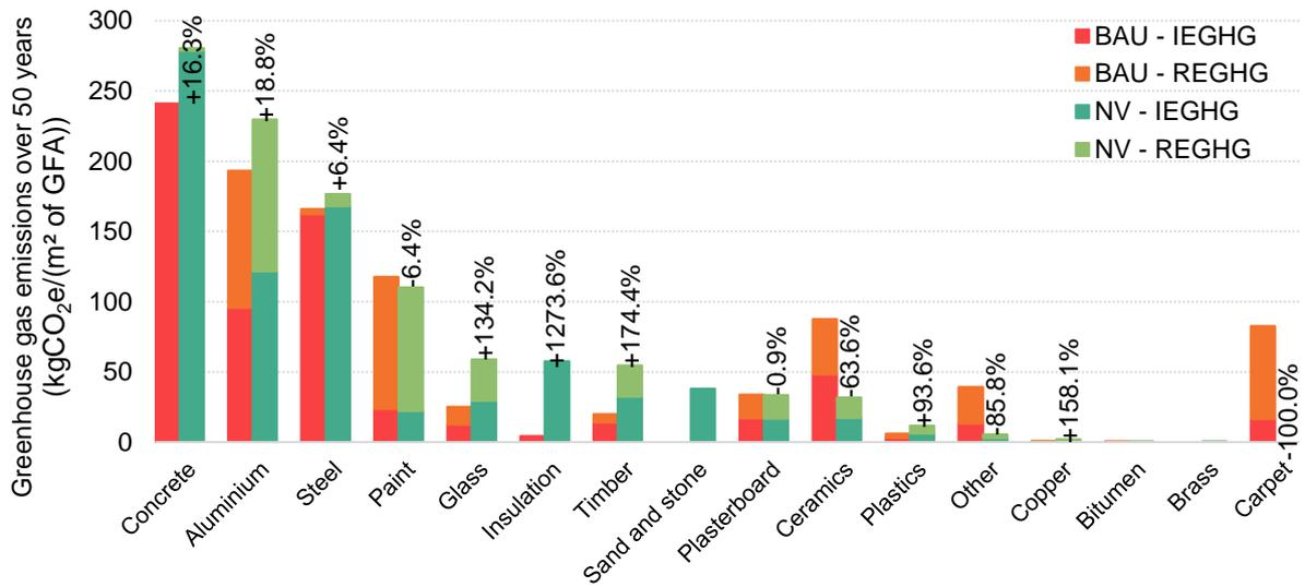
Figure 8. Initial (IEGHG) and recurrent (REGHG) life cycle embodied greenhouse gas emissions of the Nightingale Village (NV) and the business-as-usual case (BAU), in kgCO<sub>2</sub>e/(m<sup>2</sup> of gross floor area (GFA)), by material.
