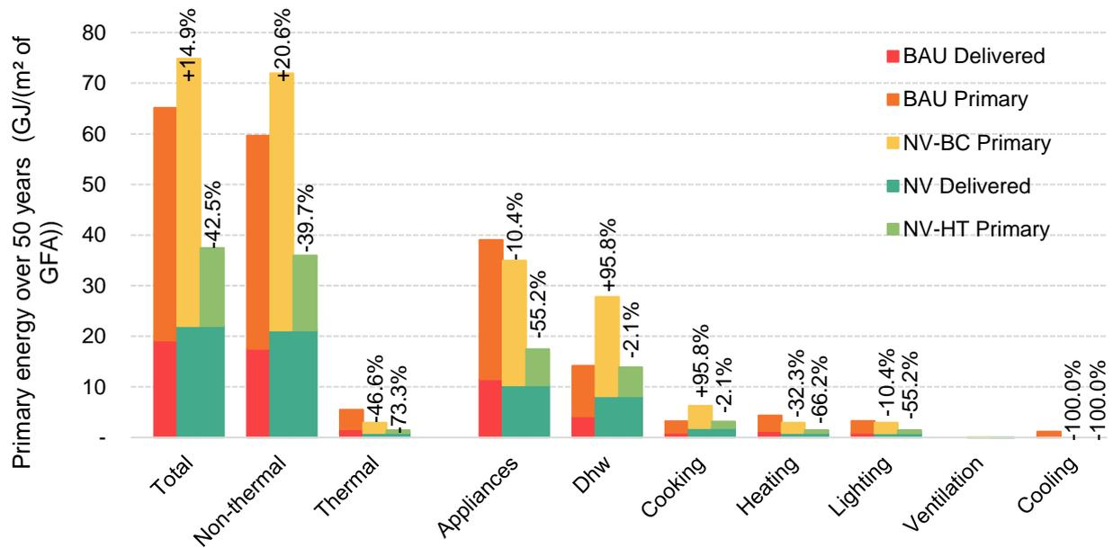
Figure 10. Delivered and primary life cycle operational energy use of the Nightingale Village scenarios (NV-BC, NV-HT) and the business-as-usual case (BAU), in GJ/m<sup>2</sup> of gross floor area, by end use.
