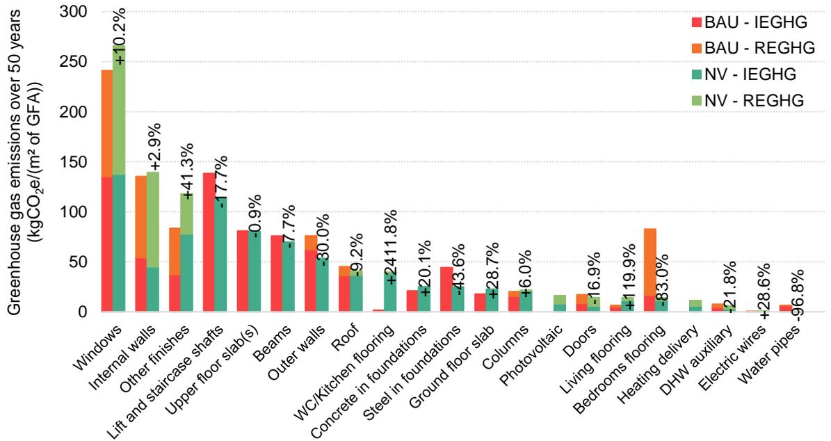
Figure 9. Initial (IEGHG) and recurrent (REGHG) life cycle embodied greenhouse gas emissions of the Nightingale Village (NV) and the business-as-usual case (BAU), in kgCO<sub>2</sub>e/(m<sup>2</sup> of gross floor area (GFA)), by assembly.
