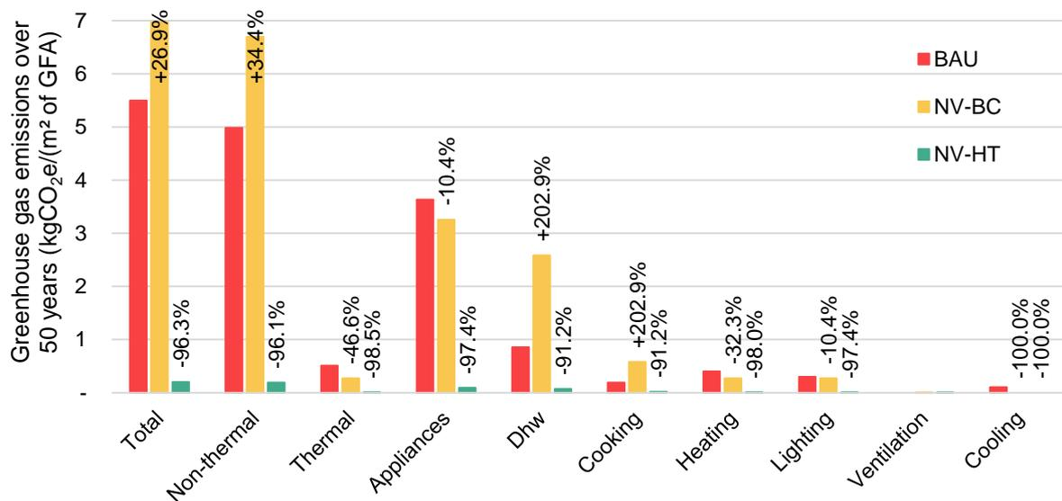
Figure 11. Life cycle operational greenhouse gas emissions of the Nightingale Village (NV) and the business-as-usual case (BAU), in kgCO<sub>2</sub>-e/m<sup>2</sup> of gross floor area (GFA), by end use.
