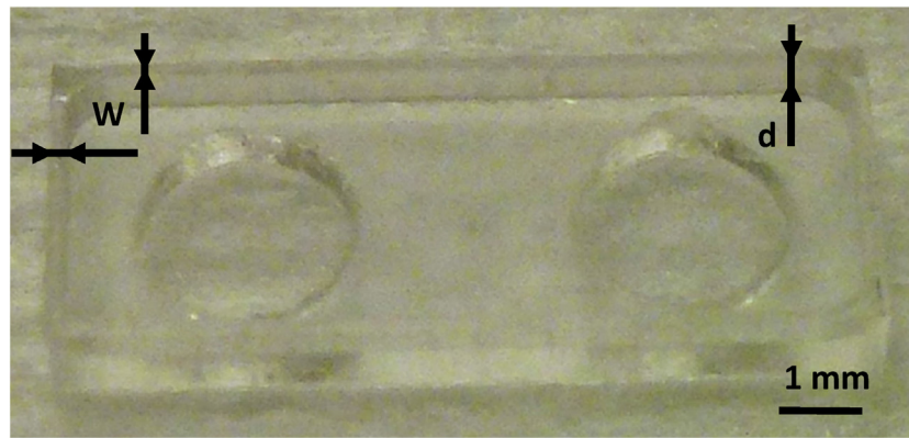
Fig. 4. Perspective view on a processed microfluidic channel. W: wall thickness and d: depth of the microfluidic channel.
