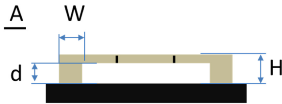
Fig. 3. Layout of the microchannel: cross-sectional view.
