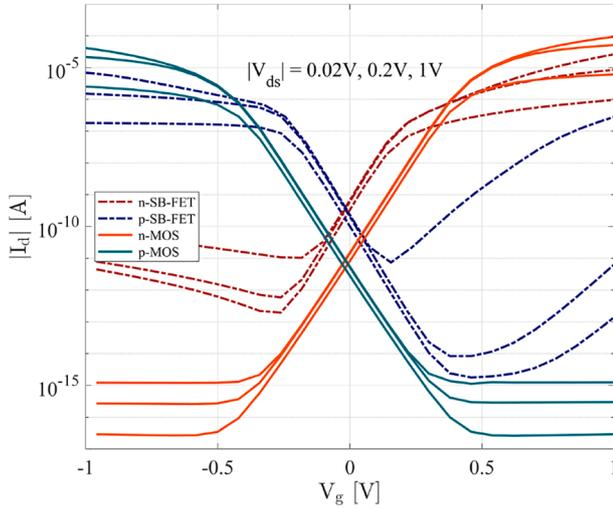
**Fig. 3.**  $I_d - V_g$  curves of CMOS with n-MOS  $L_{ch} = 200$  nm,  $W_{ch} = 1 \mu\text{m}$  & p-MOS with  $L_{ch} = 200$  nm,  $W_{ch} = 2 \mu\text{m}$ , SB-FET with n-SB-FET  $L_{ch} = 200$  nm,  $W_{ch} = 1 \mu\text{m}$  & p-SB-FET with  $L = 200$  nm,  $W_{ch} = 10 \mu\text{m}$ , for different  $V_{ds}$ .
