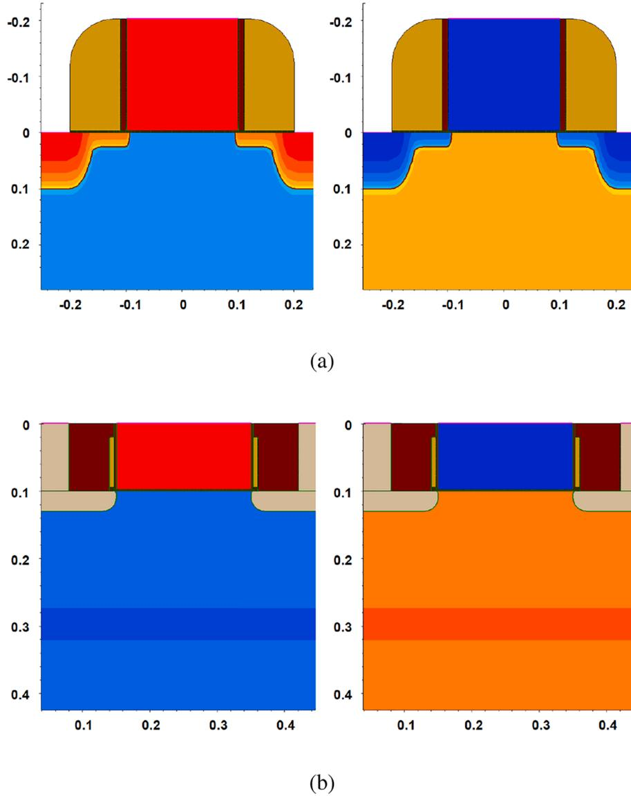
**Fig. 2.** (a) n-MOS (blue substrate)/p-MOS (orange substrate) TCAD device structures. (b) n-SB-FET (blue substrate)/p-SB-FET (orange substrate) TCAD device structures.
