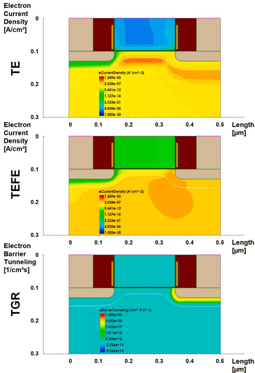
Fig. 6. p-SB-FET current densities at valley operation point  $V_D \approx 0.5$  V.
