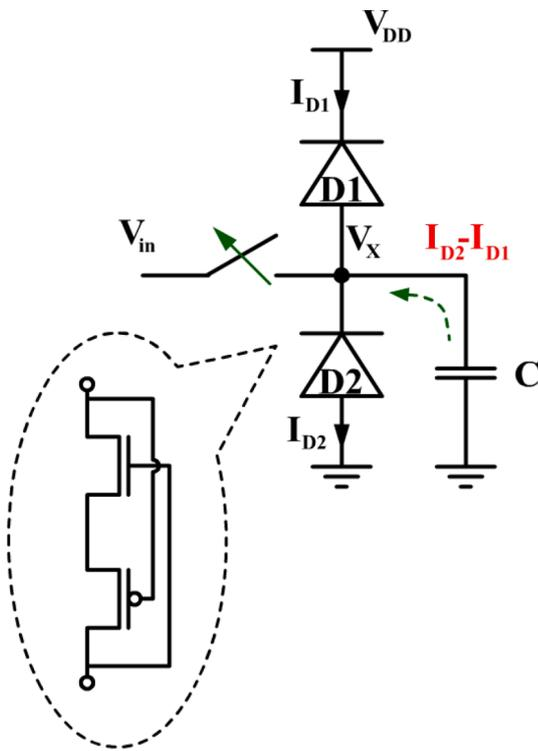
Fig. 8. ULP bistable memory cell adapted from [1].
