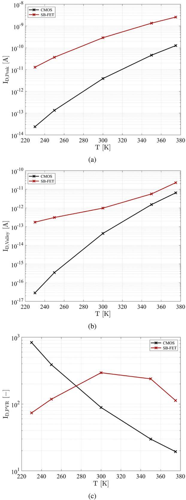
Fig. 5. (a) Peak and (b) valley  $I_D$  of CMOS vs. SB-FET ULP diode in reverse mode. (c) Peak-to-valley ratio  $I_{D,PVR}$ .
