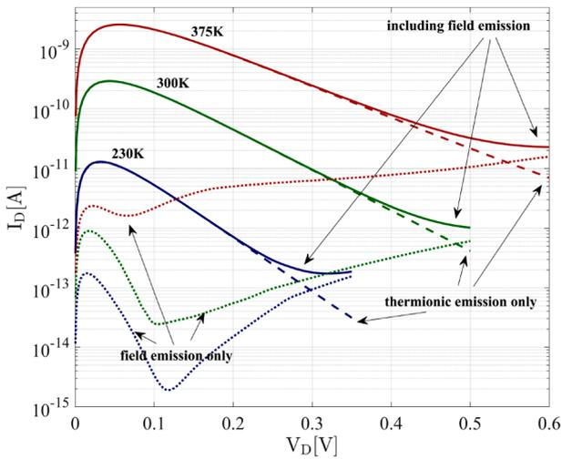
Fig. 7. SB-FET ULP diode (n-SB-FET and p-SB-FET devices) electron and hole currents with and without tunneling (field emission) over temperature for various  $|V_D|$ .
