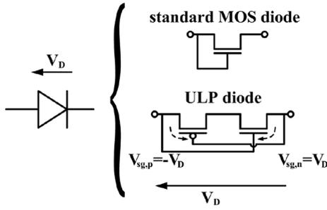
Fig. 1. Standard n-MOS diode and ULP CMOS diode architectures with forward I-V definitions adapted from [1].
