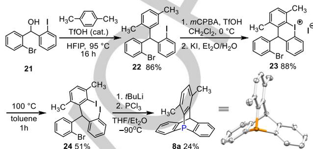
**Scheme 6.** Synthesis of the 1,4-disubstituted 9-phosphatriptycene **8a** and its X-ray structure with ellipsoid represented at the 50% level.
