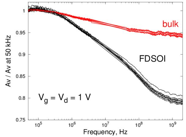
**Fig. 6:** Variation of non-normalised (top) and normalised (bottom) dimensionless voltage gain ( $g_m/g_d$ ) with frequency in bulk and FDSOI devices at  $V_g = V_d = 1.0$  V.
