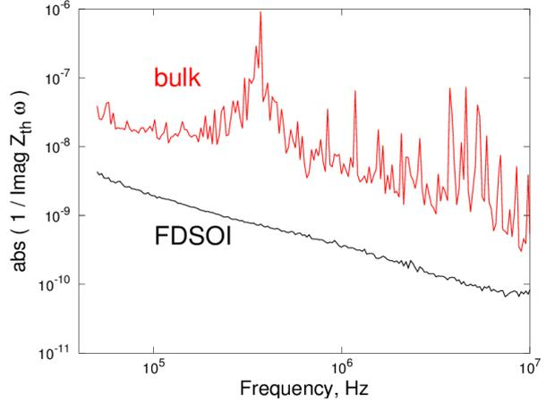
**Fig. 3:** Absolute values of the equivalent thermal capacitance  $1/\text{Imag}(Z_{th})/\omega$  as a function of frequency.
