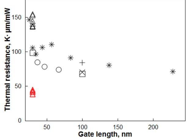
**Fig. 2:** Thermal resistance in devices of various technologies. Device details are listed in Table 1.
