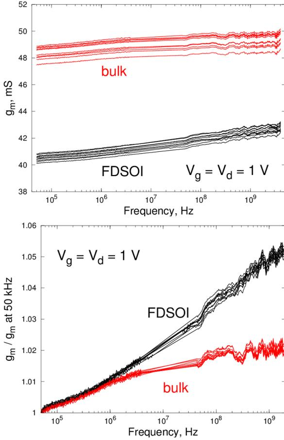
**Fig. 4:** Variation of non-normalised (top) and normalised (bottom)  $g_m$  with frequency in bulk and FDSOI devices at  $V_g = V_d = 1.0$  V.
