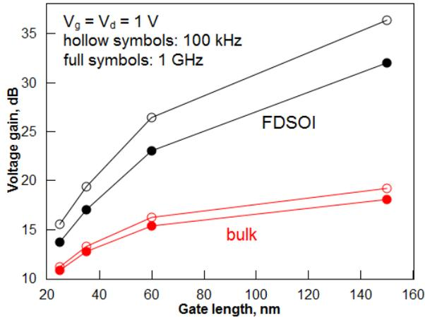
Fig. 7: Voltage gain variation with  $L_g$  at 100 kHz and 1 GHz.
