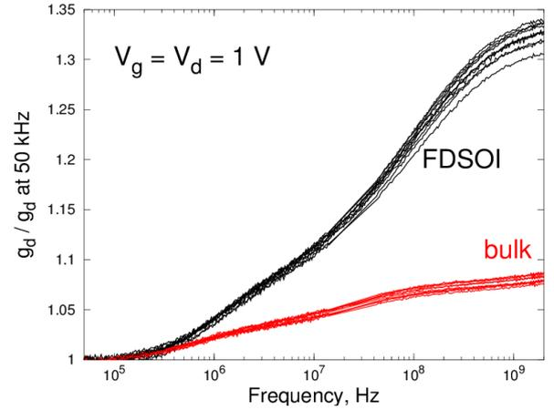
**Fig. 5:** Variation of non-normalised (top) and normalised (bottom)  $g_d$  with frequency in bulk and FDSOI devices at  $V_g = V_d = 1.0$  V.
