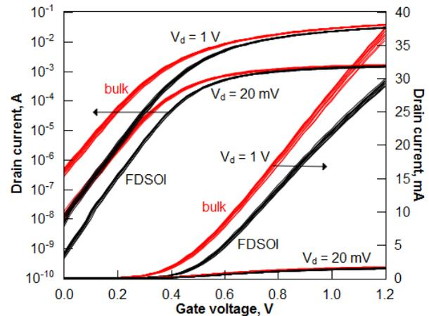
**Fig. 1:** Transfer characteristics of the studied bulk and FDSOI MOSFETs in linear ( $V_d = 20$  mV) and saturation regimes ( $V_d = 1$  V).
