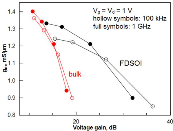
Fig. 8:  $g_m$  variation with the voltage gain in bulk and FDSOI devices with 25 - 150 nm gate lengths at 100 kHz and 1 GHz.
