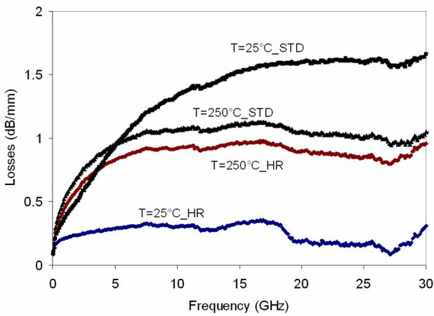
Fig.10: Measured lineic losses vs. frequency for CPW on STD and HR silicon substrates ( $W=40 \mu\text{m}$ ,  $S=24 \mu\text{m}$ ).
