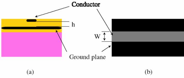
Fig. 1: MS lines: (a) cross-section and (b) top view.
