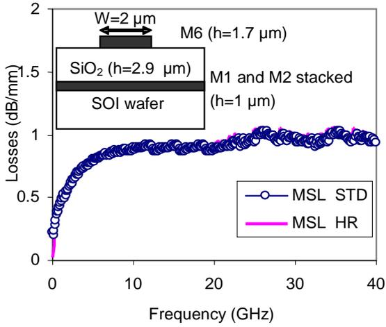
Fig. 5: Losses versus frequency for MSL lying on standard (STD, 20  $\Omega$ .cm) and high (HR, >1000  $\Omega$ .cm) SOI substrates.
