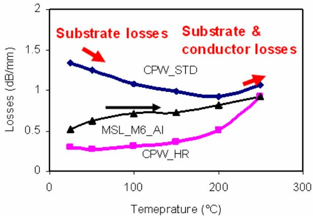
Fig.11: Comparison of measured lineic losses vs. temperature of CPW & MSL @ 10 GHz.
