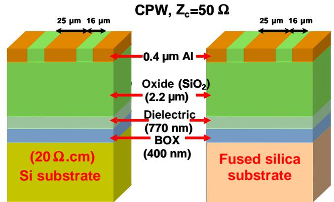
Fig. 13: 3D view of the measured transmission coplanar waveguide on standard Unibond substrate and transferred Unibond substrate on fused silica.
