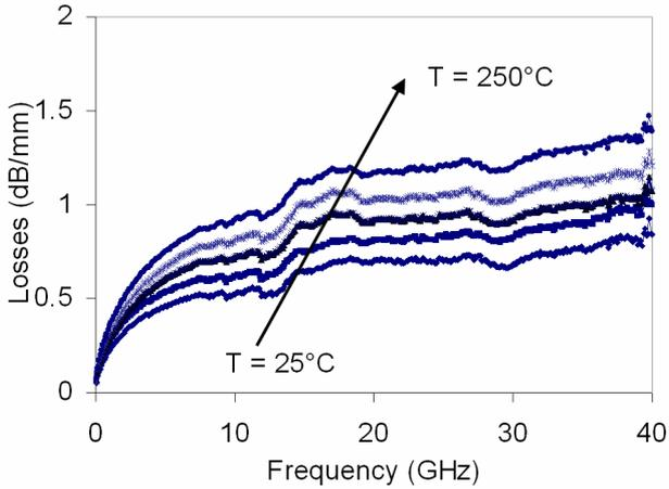
Fig.6: Measured lineic losses vs. frequency and temperature ( $W=7 \mu\text{m}$ ).
