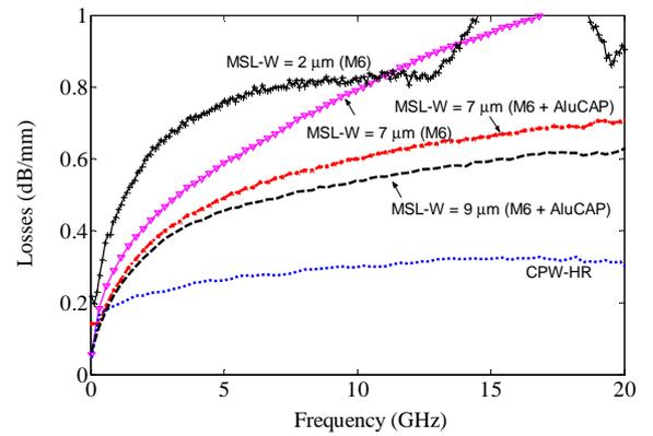
Fig. 4: Measured losses for various MSL line geometries.
