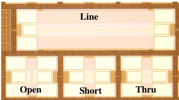
Fig. 2: Chip microphotograph of the designed MSL calibration kit.
