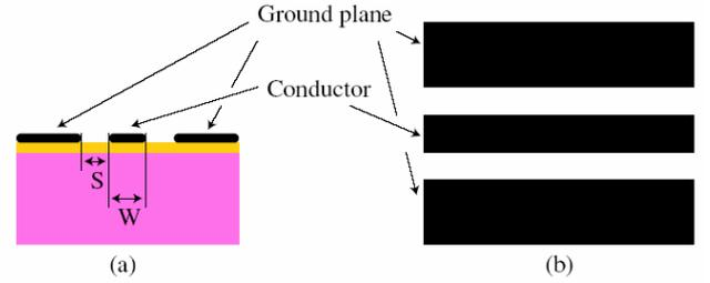
Fig. 7: CPW line: (a) cross-section and (b) Top view.
