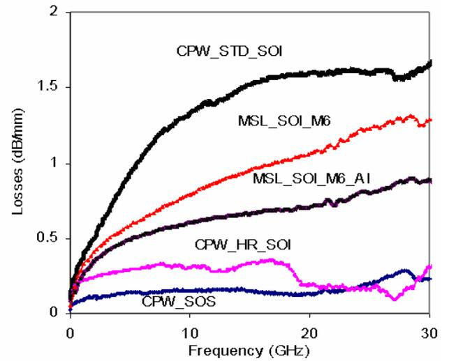
Fig. 12: Measured lineic losses of CPW on STD, HR and SOS @ room temperature.
