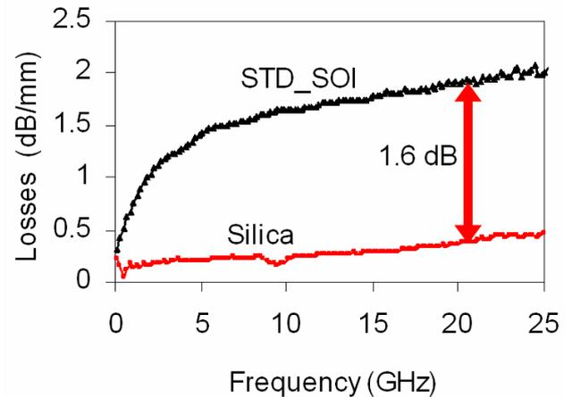
Fig. 14: Extracted attenuation on standard Unibond substrate, and transferred substrate on fused silica for the measured coplanar transmission line.
