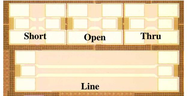
Fig. 8: Chip microphotograph of the designed CPW calibration kit.
