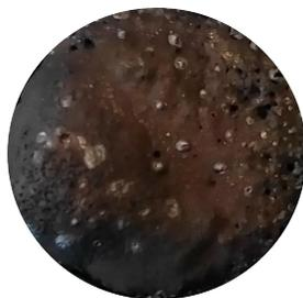
**Figure 5.10.:** Samples after plasma exposure. The change of color, probably a sign of the change in the oxidation state of iron, is visible.
