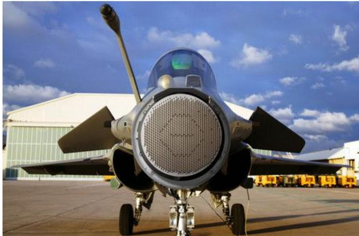
**Figure 1.1:** Active Electronically Scanned Array (AESA) on an aircraft radar [1].
