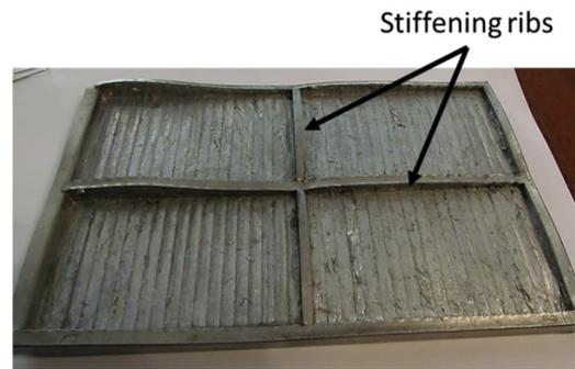
Fig. 3. Sample with stiffening ribs after the IBF process.
