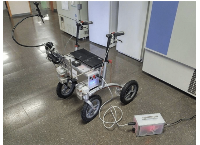
Fig. 1: Prototype FriWalk used in trials with sensors exposed.
