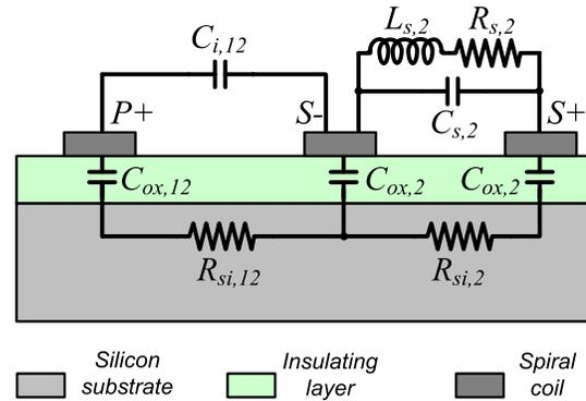
Fig. 4. Origin of parasitic elements of the on-chip transformer in silicon cross section (lumped elements of outer inductor are not represented).
