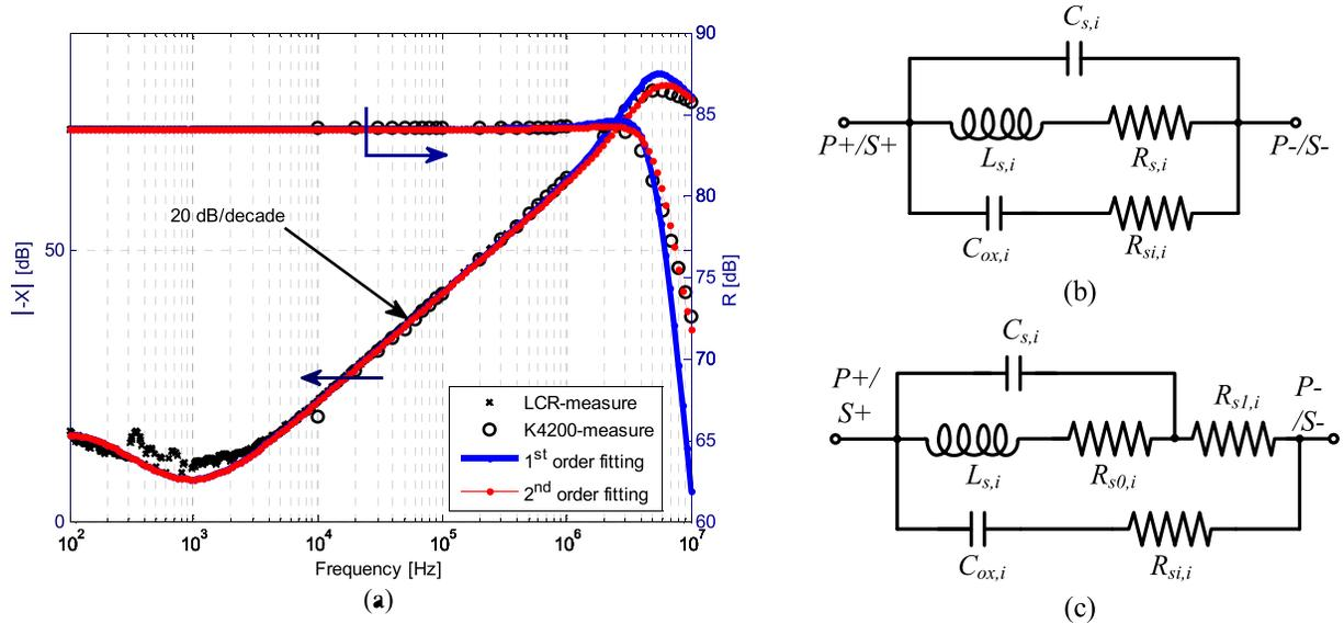
Fig. 3. (a) Inner on-chip inductor equivalent reactance (left axis) and resistance (right axis), measured and fitted curves. (b) On-chip inductor first-order lumped model. (c) On-chip inductor second-order lumped model.
