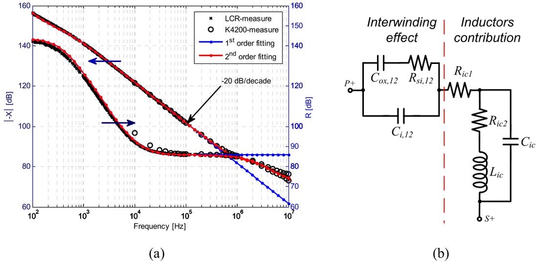
Fig. 6. Interwinding (a) reactance absolute value and resistance measured and fitted curves. (b) Equivalent electrical model.
