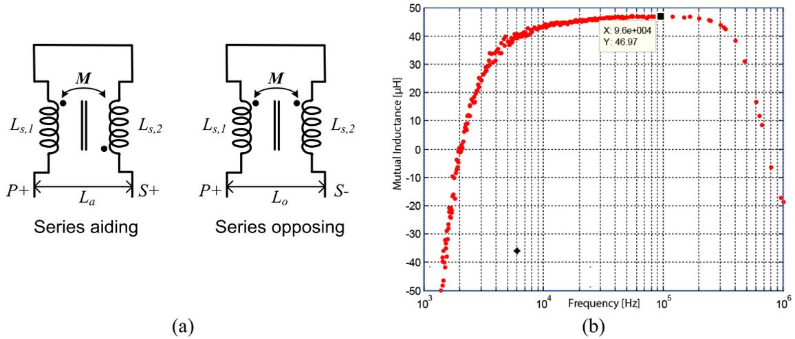
Fig. 5. (a) Inductances series-aiding and series-opposing configurations. (b) Measured mutual inductance curve.
