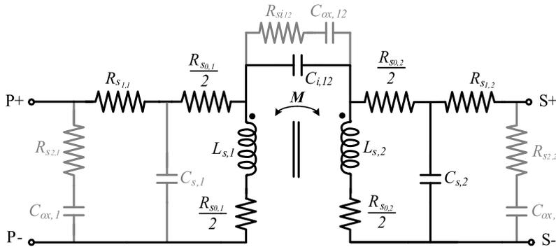
Fig. 9. Simplified lumped physical model of the tapped on-chip planar transformer (elements in gray are uninfluential).
