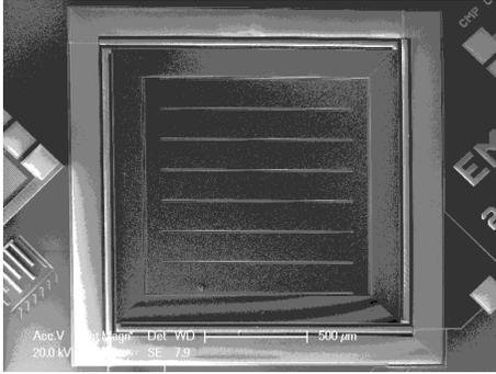
Fig. 2. Scanning electron microscope (SEM) image of the on-chip tapped transformer die.
