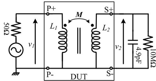
Fig. 7. Direct measurement of the transformation voltage ratio in a 3-port configuration.
