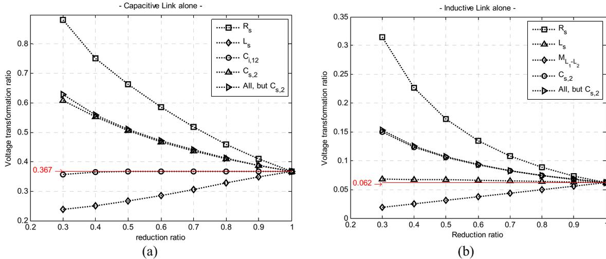
Fig. 11. On-chip lumped parameters influence on the voltage TR when considering only (a) capacitive link and (b) inductive link. (the straight line in both figures represents the initial voltage TR).
