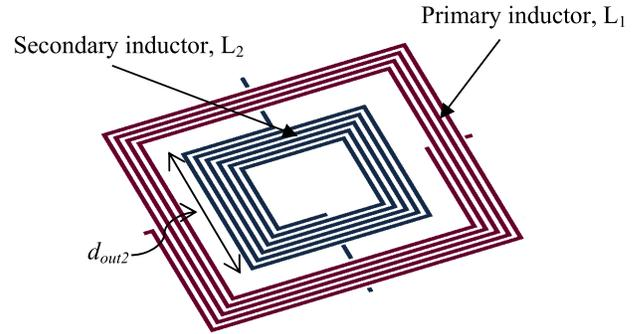
Fig. 1. Basic concept of the tapped on-chip planar transformer composed of two concentric square spirals (the number of turns is randomly set in this figure).
