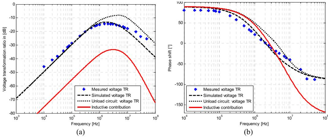
Fig. 8. Voltage TR function of the tapped on-chip transformer (a) module and (b) phase shift versus frequency.
