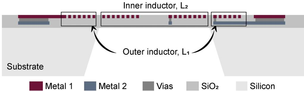
Fig. 10. Proposed structure exploiting large-size tapped transformer as MEMS-based transducer with silicon removed underneath the membrane.
