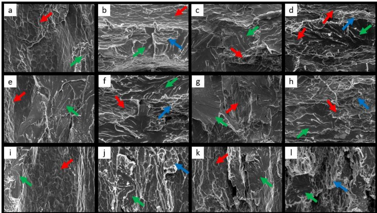
Red arrow: intergranular brittle fracture; Blue arrow: intergranular dimples;
