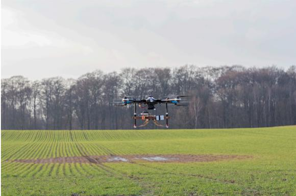
Fig. 1. Prototype drone-GPR and drone for soil moisture mapping.
