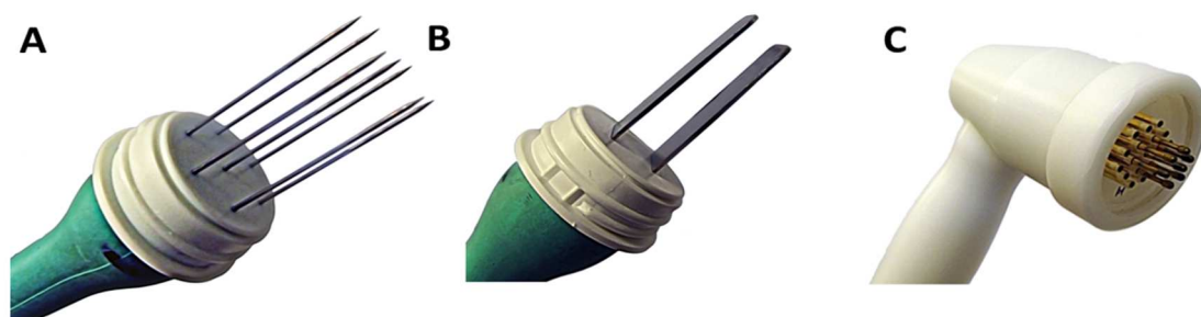
Figure 9: Different types of electrodes. A) Needle electrode; B) Plate electrode; C) Multi-electrode array. Adapted from (69).
