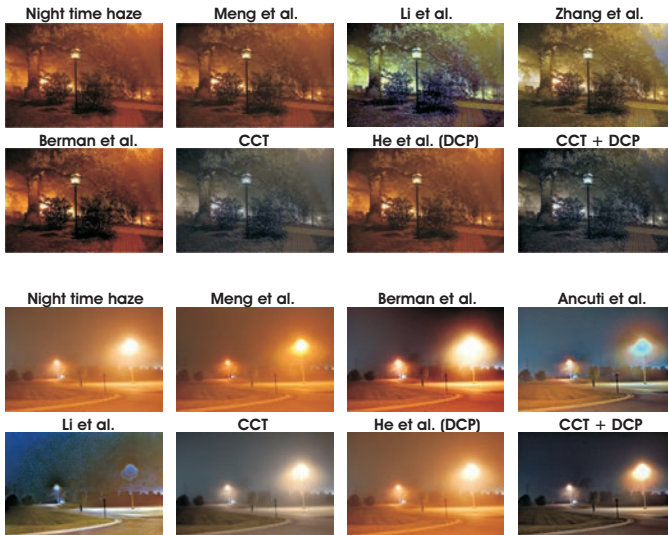
Fig. 5. Night-time image dehazing. The results of DCP applied on the images pre-processed by our CCT operator are comparable and even better than the results yielded by the local dehazing techniques of Ancuti et al. [17] and Berman et al. [36].
