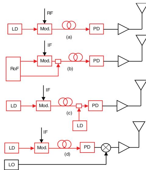
Fig. 1. Fiber transports of broadband mobile signals: (a) RoF; (b) optical self-heterodyne; (c) optical heterodyne; (d) IFoF system. LD: laser diode, Mod: modulator, PD: photodiode, LO: local oscillator, RoF: radio-over-fiber, IFoF: intermediate frequency-over-fiber.
