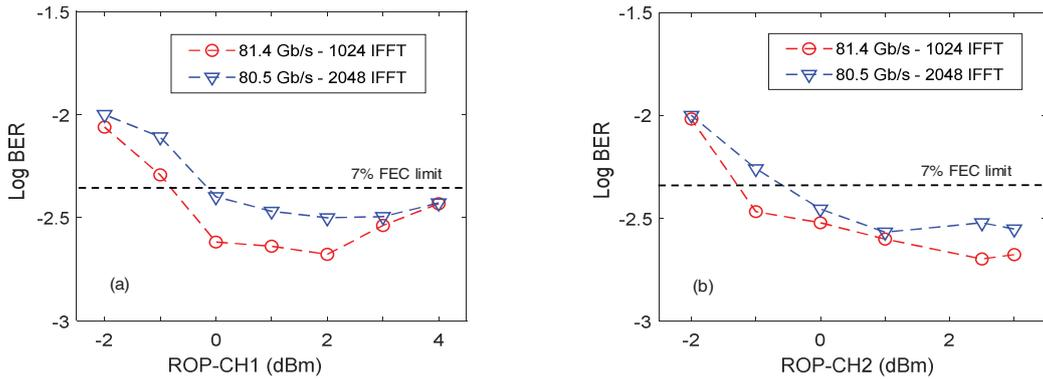
Fig. 5. Performance of the 2×2 MIMO fiber–wireless system: (a) versus received optical power in channel 1; (b) versus received optical power in channel 2.
