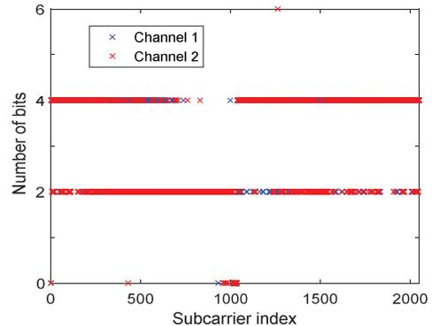
Fig. 4. Bit loading for the  $2 \times 2$  MIMO signal using 2048 subcarriers.
