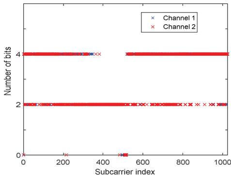
Fig. 3. Bit loading for the  $2 \times 2$  MIMO signal using 1024 subcarriers.
