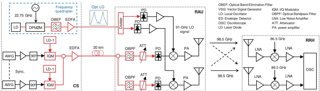
Fig. 2. Experimental setup for the  $2 \times 2$  MIMO fiber-wireless system in the W band using an IFoF transmission.
