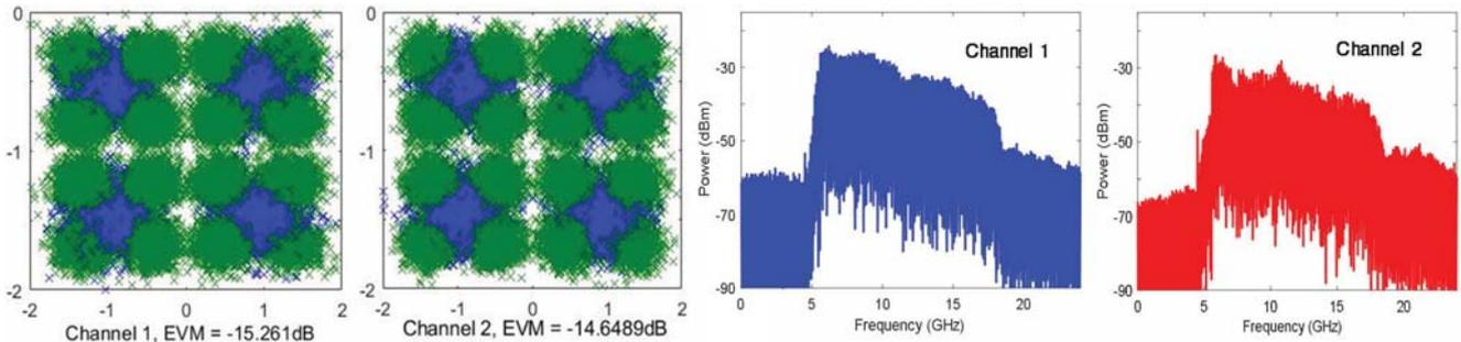
Fig. 6. Examples of received constellations and spectrums of the 81.4 Gb/s signal using 1024 subcarriers.
