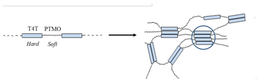
Figure 6.2: Schematic illustration of TPE chains association through crystallization of HSs.
