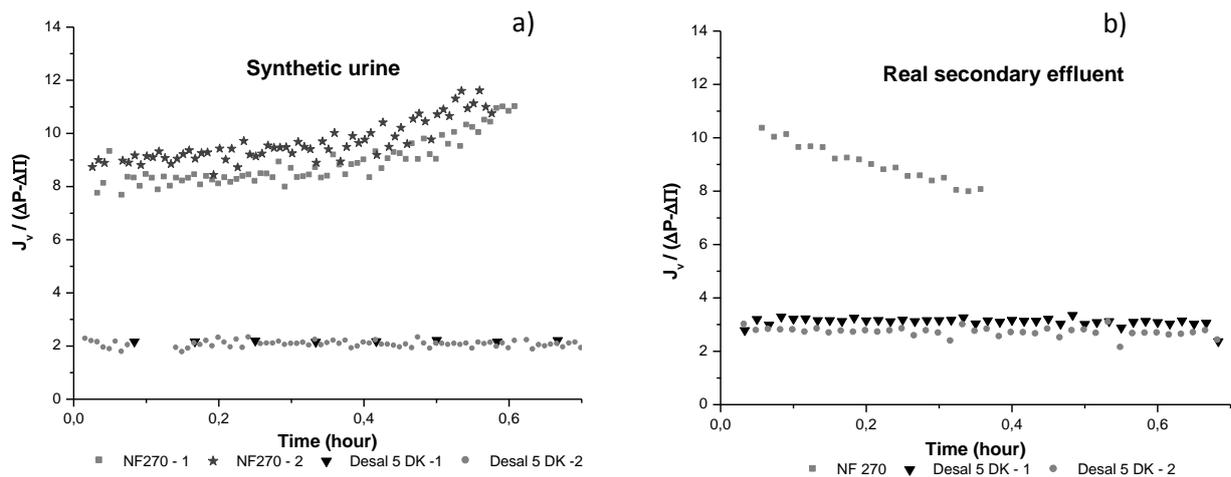
369 Figure 2 Membrane permeance considering the osmotic pressure difference ( $\Delta\pi$ ) evolution during the nanofiltration experiment with
