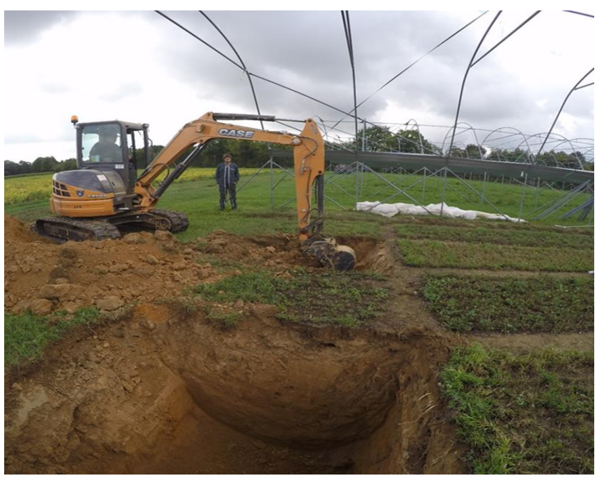
Fig 4. Digging of the pits in front of the parcels (left), placement of a grid (center), root countings in each cell of the grid (right). Each cell was a square of 2.5cm by 2.5cm. The measures were taken on a width of 1.5m and a depth of 1.5m.
