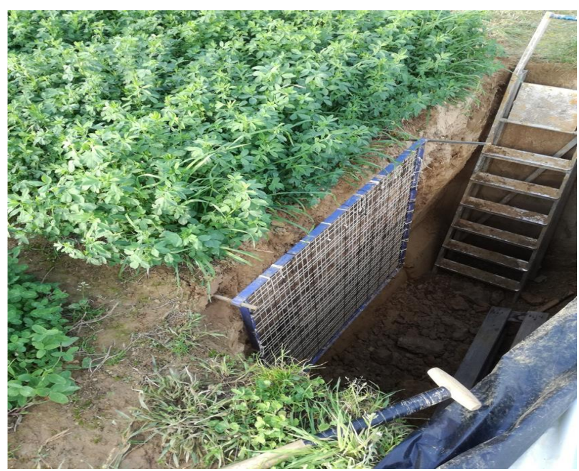
Fig 4. Digging of the pits in front of the parcels (left), placement of a grid (center), root countings in each cell of the grid (right). Each cell was a square of 2.5cm by 2.5cm. The measures were taken on a width of 1.5m and a depth of 1.5m.
