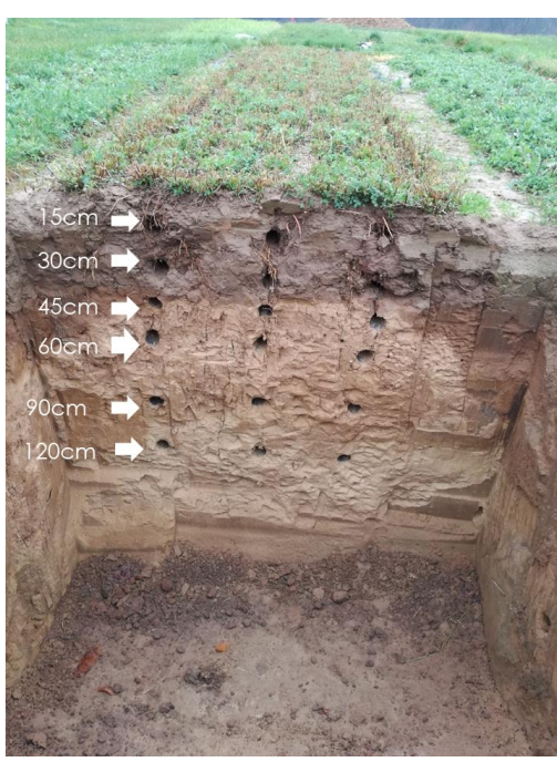
Fig 5. Position of the horizontal samples (left) and vertical sampling (right). The horizontal samples were taken at the depths indicated on the image and with 3 repetitions. The vertical samples were taken at the 4 corners of a square of 90cm of size.
