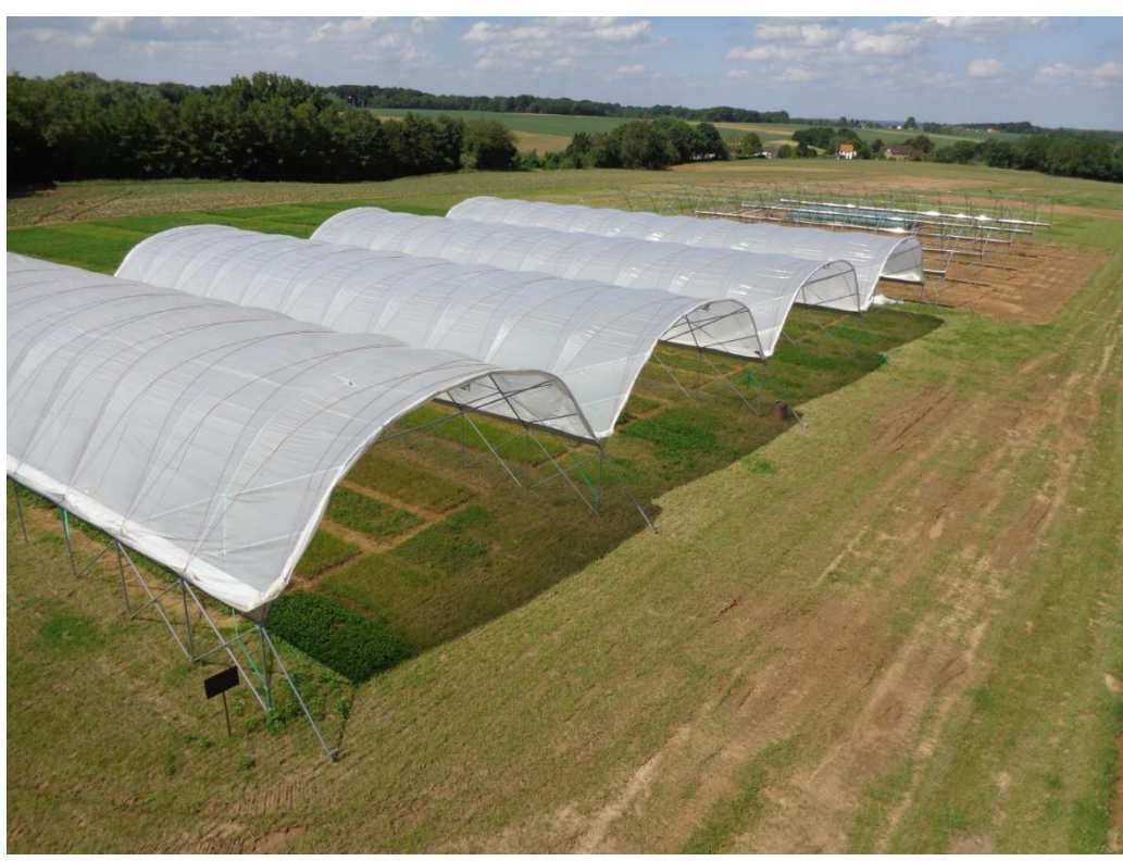
Fig 1. Aerial view of the parcels of the Fordrought project. The plastic covers above the parcels enable to enforce a water deficit.
