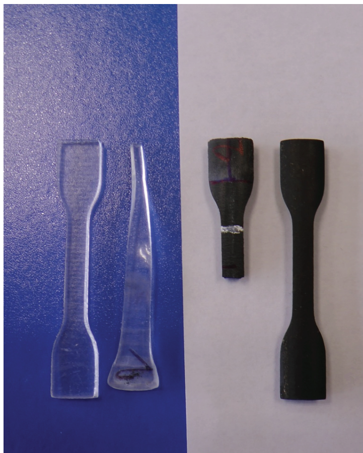
Figure 4.2: Necking behaviour observed in neat polymer aged to low dose (white samples). The total recovery in industrial EPDM (black samples).
