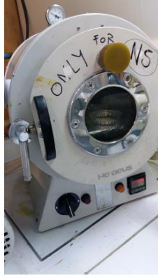
Figure 2.20: The oven for drying the swollen sample used in this study.
