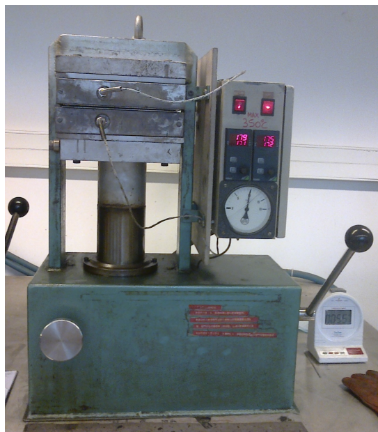
Figure 2.3: The machine for pellet melting and forming of polymer sheet.
