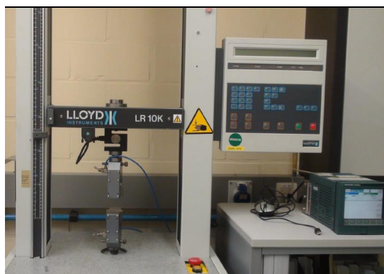
Figure 2.7: The Lloyd LR10K tensile machine.
