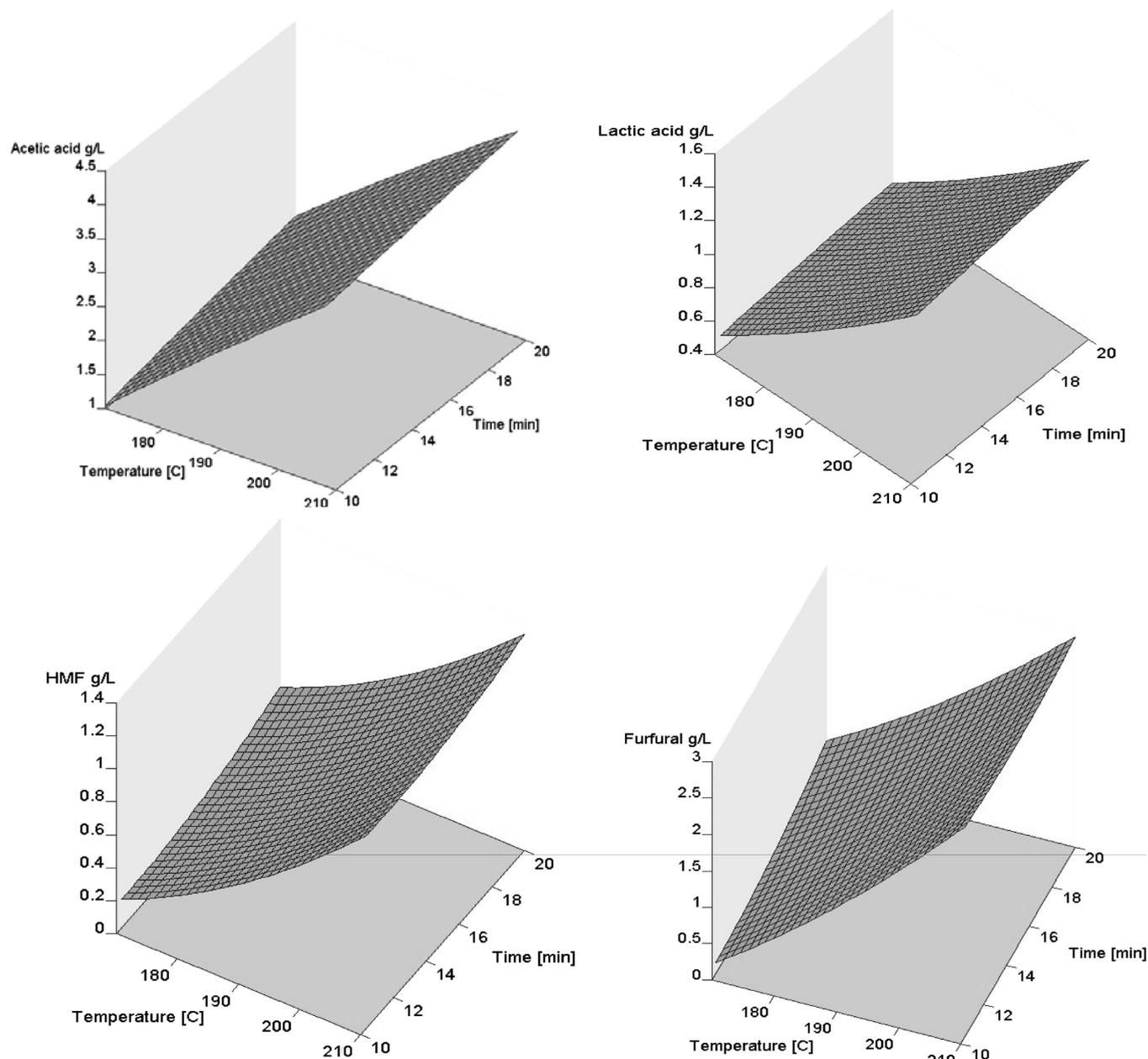
**Figure 9.** Response surfaces for the byproducts: acetic acid, lactic acid, HMF, and furfural (filtrate).
