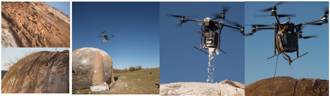
Figure. 2: From Left to Right Close ups on the matter surface adhesion and the drone spraying 2 kinds of clay mix over the formwork. January 2018. Test at the Barcelona drone center by the authors.
