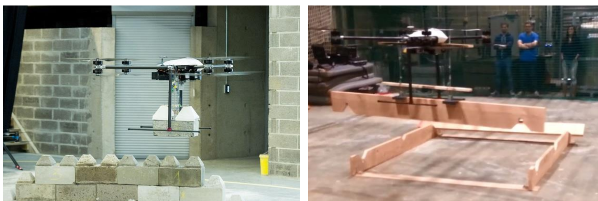
Figure 1: The drone used for the lab tests (Drone Zone UCLouvain/Belgium). On the left: assembling of masonry elements. On the right: assembling of timber beams.
