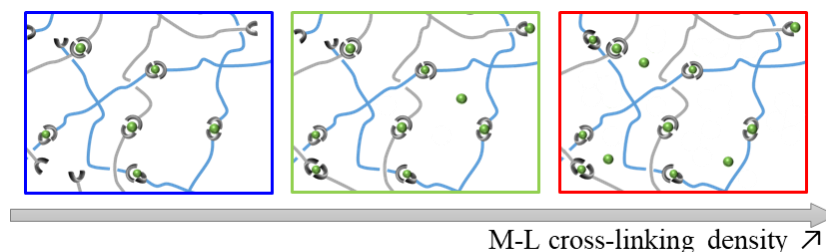
Figure 5.12 Schematic view of metallo-supramolecular networks obtained from telechelic 4-arm star precursor, highlighting the influence of physical cross-linking density.
