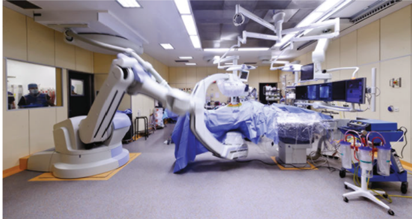
Fig. 1. Panoramic view of our operating room equipped with the Artis Zeego (robotic C-arm fluoroscopy), its synchronized translucent table (covered by sterile drapes) and different control screens
