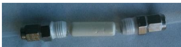
Figure 3. Picture of the plug flow reactor applied for a continuous biocatalytic transamination reaction. The functionalised silica monolith is casted into a heat-shrinkable Teflon tube and both ends are respectively connected to (i) a syringe pump and (ii) a sample collector. The transaminase was immobilised by covalent grafting using glutaraldehyde as a coupling agent. [25]
