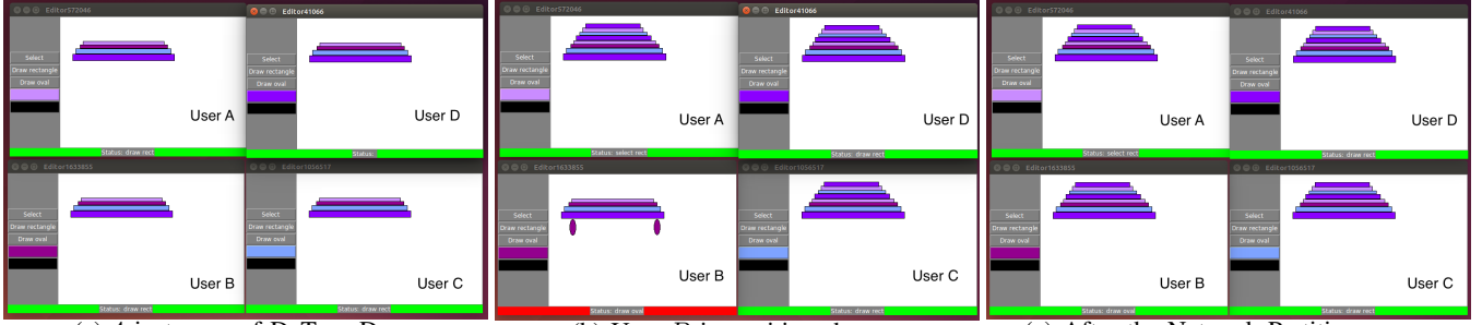
(a) 4 instances of DeTransDraw (b) User B is partitioned-away (c) After the Network Partition ceases Figure 6: DeTransDraw facing Network Partition. (a) Suppose users A , B , C and D , where B is partitioned away. (b) During the partition the canvas across the partitions diverges with time. (c) When the partition ceases, the application, being self-adaptive and self-optimized, syncs based on the observed phase transitions, and achieves the canvas consistency and full functionality.
