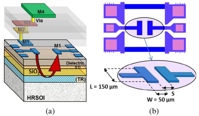
Fig. 10. Crosstalk structure in 0.18 μm TowerJazz CMOS process: (a) schematic; (b) top layout view.
