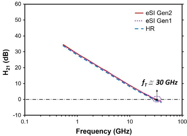
**Fig. 4.** Current gain cutoff frequency  $f_T$  at  $V_{DS} = 1.2$  V and  $V_{GS}$  at which  $g_m$  (transconductance) is maximum for body-tied RF transistor for 3 different wafers of 1st generation of trap-rich high resistivity SOI (eSI Gen1), 2nd generation of trap-rich high resistivity SOI (eSI Gen2) and high resistivity SOI (HR).
