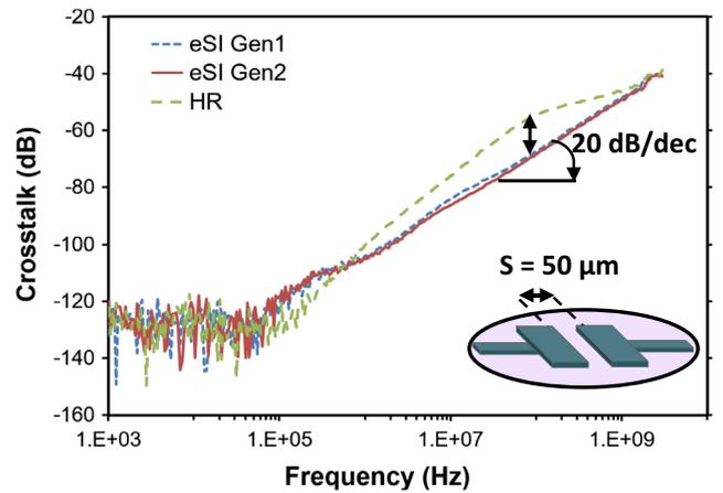
Fig. 11. Measured crosstalk versus frequency on HR-SOI, eSI Gen1 and eSI Gen2 HR-SOI substrates for a crosstalk structure with a pad distance of S = 50 μm and zero substrate bias.
