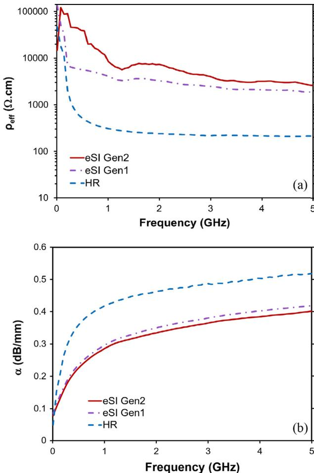
Fig. 7. (a) Effective resistivity, (b) Total Loss (Conductor and substrate) of 3 different substrates of 1st generation of trap-rich high resistivity SOI (eSI Gen1), 2nd generation of trap-rich high resistivity SOI (eSI Gen2) and high resistivity SOI (HR).
