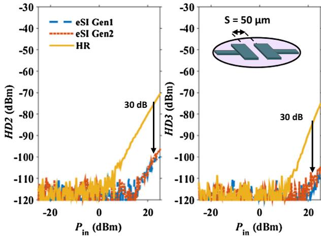
Fig. 12. Measured 2nd (HD2) and 3rd (HD3) harmonic distortions of a crosstalk structure with a pad distance of  $S = 50 \mu\text{m}$  and zero DC substrate bias.
