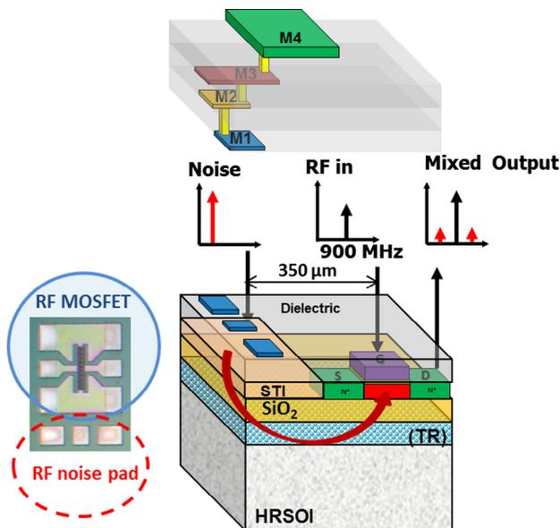
Fig. 13. Cross-section of PD SOI nMOSFET with a noise pad at a distance of  $350 \mu\text{m}$  (center to center) lying on either eSI HR-SOI or HR-SOI wafers when a trap-rich layer exists or not respectively.
