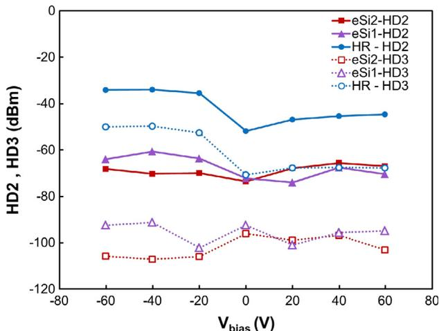
Fig. 9. The variation of 2nd harmonic distortion (HD2) and 3rd harmonic distortion (HD3) with bias changing from -60 V to +60 V at input power P<sub>in</sub> = 20 dBm for 3 different wafers: 1st generation of trap-rich high resistivity SOI (eSI Gen1), 2nd generation of trap-rich high resistivity SOI (eSI Gen2) and high resistivity SOI (HR).
