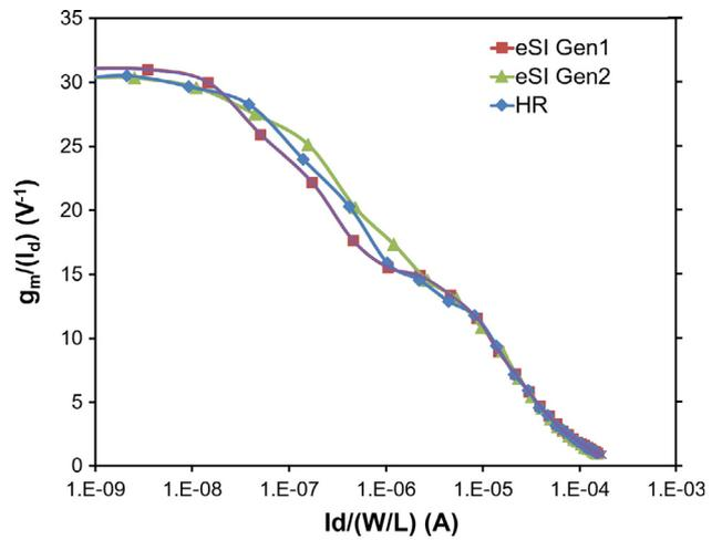
Fig. 3.  $g_m/I_D$  ratio versus  $I_D/(W/L)$  DC transistor in linear regime ( $V_{\text{DS}} = 50 \text{ mV}$ ) on 3 different wafers of 1st generation of trap-rich high resistivity SOI (eSI Gen1), 2nd generation of trap-rich high resistivity SOI (eSI Gen2) and high resistivity SOI (HR).
