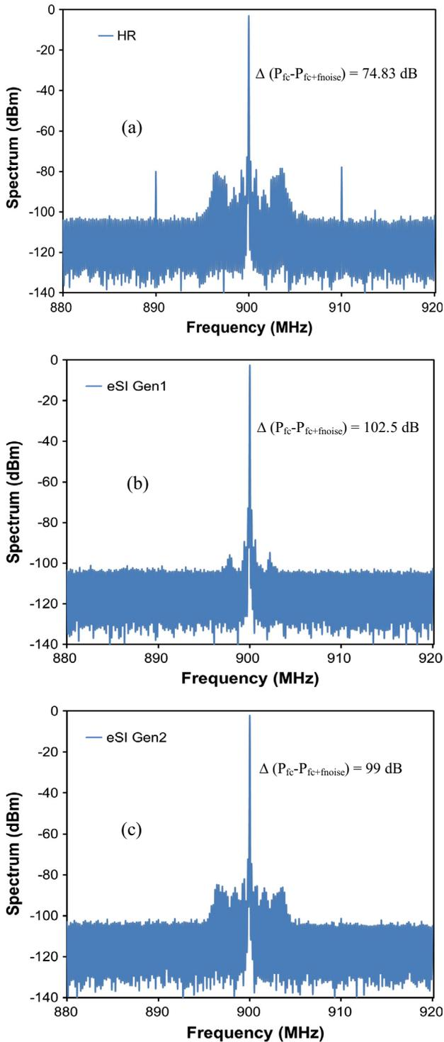
**Fig. 15.** Output spectrum of measured fundamental and noise signal at the drain port of the PD nMOSFET having a gate length ( $L_g$ ), gate finger width ( $W_f$ ) and number of the finger ( $N_f$ ) of 0.24  $\mu\text{m}$ , 2  $\mu\text{m}$  and 64 respectively biased in saturation with a 900 MHz fundamental RF signal at the gate. A digital noise signal (5 V peak-to-peaks at 10 MHz) is injected to the RF noise pad on (a) HR-SOI, (b) eSI Gen1 HR-SOI and (c) eSI Gen2 HR-SOI substrates.
