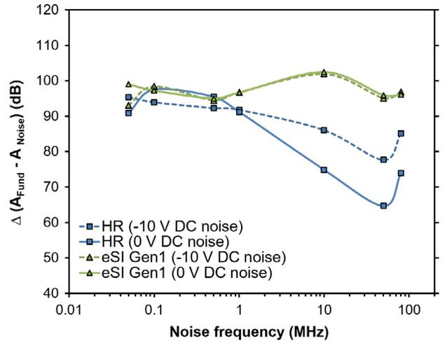
**Fig. 16.** Power level difference between 900 MHz fundamental RF input ( $A_{\text{Fund}}$ ) and digital noise signal ( $A_{\text{Noise}}$ ) on HR-SOI and eSI Gen1 substrates.
