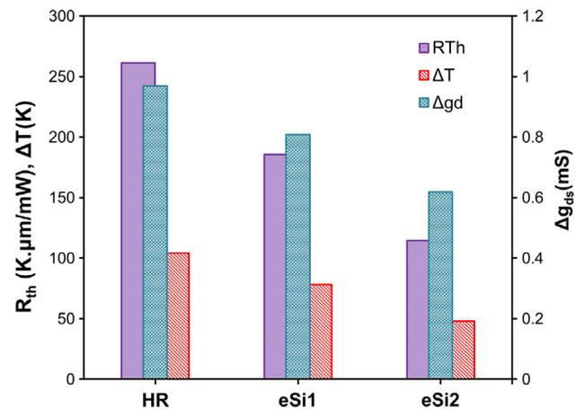
**Fig. 6.** Average temperature rise ( $\Delta T$ ), thermal resistance ( $R_{th}$ ) and output conductance transition amplitude due to self-heating ( $\Delta g_{ds}$ ) in studied body-tied RF transistors biased at  $V_{GS} = V_{DS} = 1.4$  V for 3 different wafers of 1st generation of trap-rich high resistivity SOI (eSI Gen1), 2nd generation of trap-rich high resistivity SOI (eSI Gen2) and high resistivity SOI (HR).
