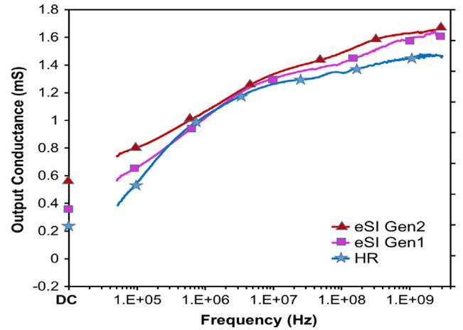
**Fig. 5.** Output conductance ( $g_{ds}$ ) variation with frequency at  $V_{gs} = V_{ds} = 1.4$  V.
