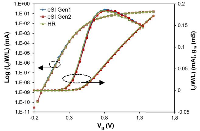
Fig. 2. Normalized  $I_D$ - $V_G$  (linear and logarithmic) and  $g_m$ - $V_G$  characteristics in linear regime ( $V_{\text{DS}} = 50 \text{ mV}$ ) of DC transistor for 3 different wafers of 1st generation of trap-rich high resistivity SOI (eSI Gen1), 2nd generation of trap-rich high resistivity SOI (eSI Gen2) and high resistivity SOI (HR).
