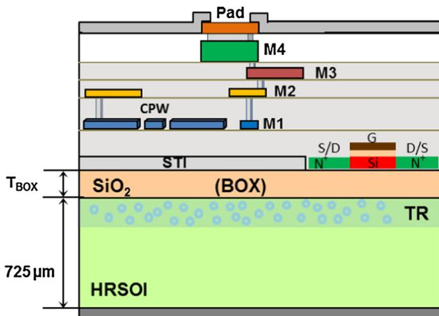
Fig. 1. Cross-section details of 4-metal layer 0.18  $\mu\text{m}$  SOI CMOS process by TowerJazz on top of high resistivity SOI substrates having different BOX thickness ( $T_{\text{BOX}}$ ) provided by SOITEC.
