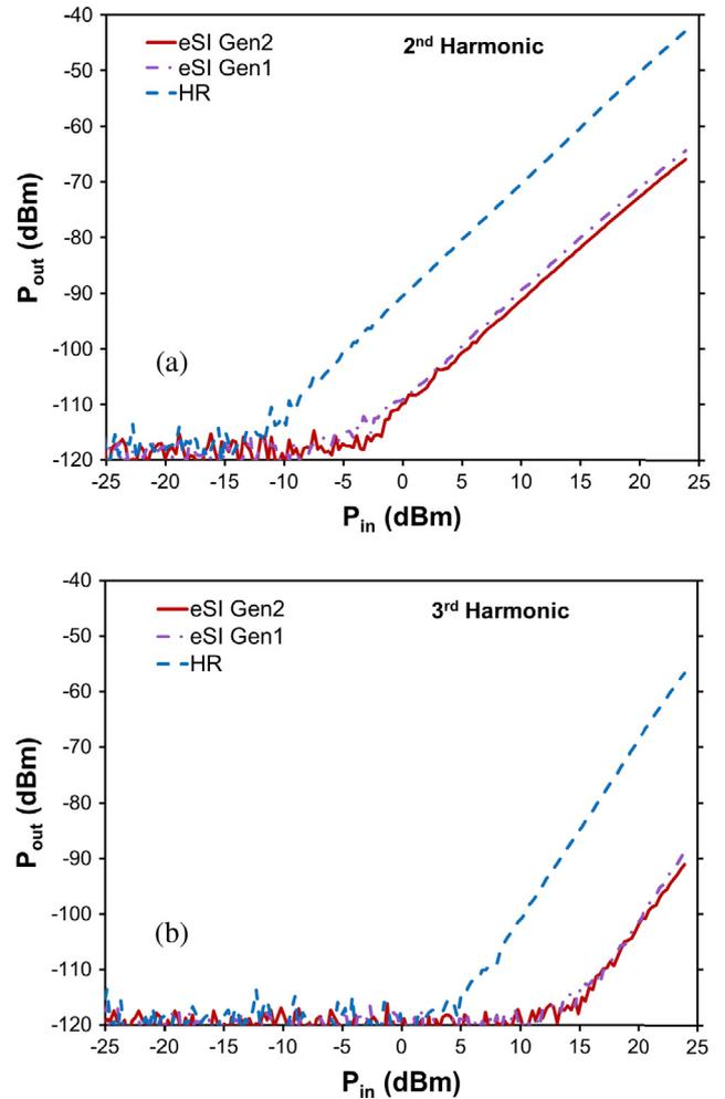
Fig. 8. (a) 2nd and (b) 3rd harmonic distortion measured at zero bias by CPW lines on 3 different wafers: 1st generation of trap-rich high resistivity SOI (eSI Gen1), 2nd generation of trap-rich high resistivity SOI (eSI Gen2) and high resistivity SOI (HR).
