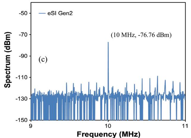
Fig. 14. Frequency spectrum of measured noise signal at the drain port of the PD nMOSFET having a gate length ( $L_g$ ), gate finger width ( $W_f$ ) and number of the finger ( $N_f$ ) of  $0.24 \mu\text{m}$ ,  $2 \mu\text{m}$  and 64 respectively biased in saturation with no fundamental RF signal at the gate. A digital noise signal (5 V peak-to-peaks at 10 MHz) is injected to the RF noise pad on (a) HR-SOI, (b) eSI Gen1 HR-SOI and (c) eSI Gen2 HR-SOI substrates.
