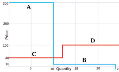
Figure 1.1: Instance with a 'non-convex bid' C - start up cost or min. power output
