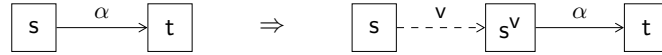
Figure 4.12. Transition mapping for HVS to HMI-LTS translation for non- \tau transitions. The transition from the original system model (on the left) induces two transitions in the expanded system model (on the right), where v = \mathcal{O}(s) .
