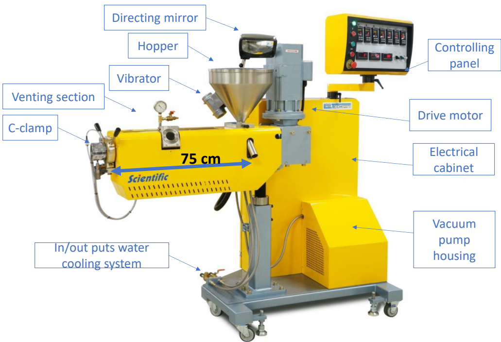
Figure S2 LabTech single screw extruder (1) (Model: LE25-30/CV, Thailand)
