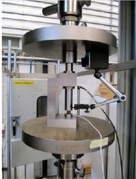
Figure 2.15: Experimental setup of the compressions tests.
